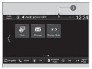
**2.** A notification icon is continuously displayed in the header area until the new message is read.
