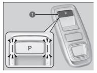
The shift position changes to  $\boxed{\textbf{P}}$  when you press the  $\boxed{\textbf{P}}$  button while the vehicle is parked with the power mode in ON. The indicators on the sides of the  $\boxed{\textbf{P}}$  button come on.
