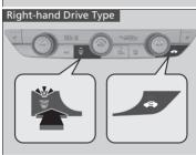
Pressing the (windscreen demister) button turns the air conditioning system on and automatically switches the system to fresh air mode.
