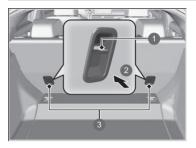
A tether anchorage point is provided behind each rear outer seating position.
