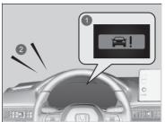
The system provides visual and audible alerts of a possible collision, and stops if the collision is avoided.
