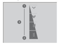
The default deceleration stage is w. Each paddle selector operation makes a single stage deceleration change.
