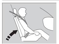
Adjust the driver's seat-back to a comfortable, upright position, leaving ample space between your chest and the airbag cover in the centre of the steering wheel.
