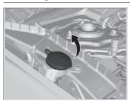
Check the amount of window washer fluid by looking at the reservoir.
