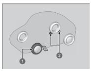
**5.** Place a wheel block or rock in front and rear of the wheel diagonal to the flat tyre.
