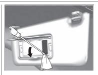
**2.** Remove the old bulb and insert a new bulb.
