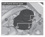
The fluid level should be between the **MIN** and **MAX** marks on the side of the reserve tank.
