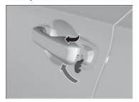
Pull and hold the outer handle. Insert the built-in key into the key cylinder from below the handle and then turn it.
