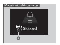
If no vehicle is ahead of you before you resume driving, depress the accelerator pedal and ACC with Low Speed Follow will operate again within the prior set speed.
