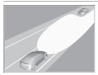
When driving at night, the front wide view camera detects light sources such as street lights or the lights of an oncoming or preceding vehicle. The system automatically switches the headlights between low and high beam depending on the situation. In addition, the system automatically adjusts the light distribution of the high beams in order to reduce glare for preceding and oncoming vehicles.
