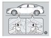
**1.** Place the jack under the jacking point closest to the tyre to be changed.
