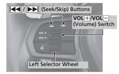
● VOL+/VOL- (Volume) Switch Press to adjust the volume up/down.
