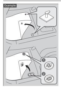
The driver's floor mat hooks over floor anchorages, which keep the mat from sliding forward.
