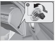
Passenger Front Airbag ON/ OFF Switch
