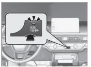
The rear demister and heated door mirrors automatically switch off after 10-30 minutes depending on the outside temperature. However, if the outside temperature is 0°C or below, they do not automatically switch off.
