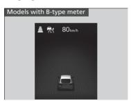
While driving down steep hills, ACC with Low Speed Follow brakes to inhibit excessive acceleration for maintaining the set speed. However, the vehicle speed may become faster than the set speed.
