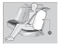
Deployed Side Airbag
