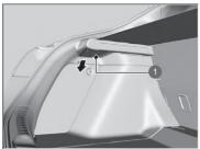
**1.** Open the hatch and remove the cover on the left side of luggage area.
