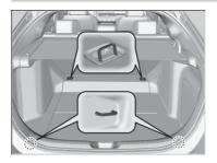
The tie-down anchorages on the luggage area floor can be used to install a net for securing items.
