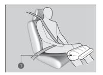
Deployed Passenger's Knee Airbag
