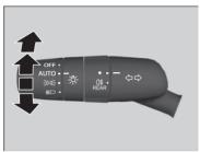
The exterior lights will switch on automatically when the light switch is set to **AUTO** while the power mode is in ON.
