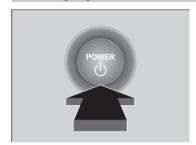
If you carry the keyless remote and press **POWER** button without depressing the brake pedal, the power mode will change in this order: VEHICLE OFF→ACCESSORY→ON→ VEHICLE OFF.
