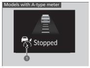
Your vehicle also stops automatically. The **Stopped** message appears on the gauge. When the vehicle ahead of you starts again, if you press the **RES/+/SET/-** switch up or down, or depress the accelerator pedal, ACC with Low Speed Follow operates again within the previously set speed.
