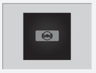
If the driver does not grip the steering wheel after the warning above has repeatedly appeared, a warning buzzer will sound and Traffic Jam Assist will be cancelled.
