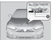
3. Push the bonnet latch lever (located under the front edge of the bonnet to the centre) to the side and raise the bonnet. Once you have raised the bonnet slightly, you can release the lever.
