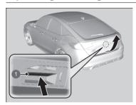
When all the doors are unlocked or you press the hatch unlock button on the remote transmitter, the hatch is unlocked. Press the hatch release button and lift open the hatch.
