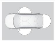
When you carry the keyless remote, you can lock/unlock the doors, fuel fill door and hatch. You can lock/unlock the doors, fuel fill door and hatch within a radius of about 80 cm (32 inches) from the outside door handle or hatch release button.
