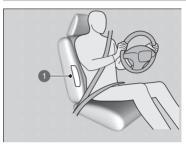
The centre airbag is housed in the centre side of the driver's seat-back.
