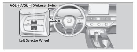
**Left Selector Wheel:** Roll up or down to select **Phone** on the driver information interface, and then press the left selector wheel.
