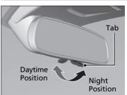
Flip the tab to switch the position.
