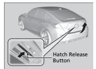
When all the doors are unlocked or you press the hatch unlock button on the remote transmitter, the hatch is unlocked. Press the hatch release button and lift open the hatch.
