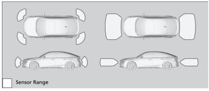
The sonar sensors are situated in the front and rear bumpers, and the front grille.
