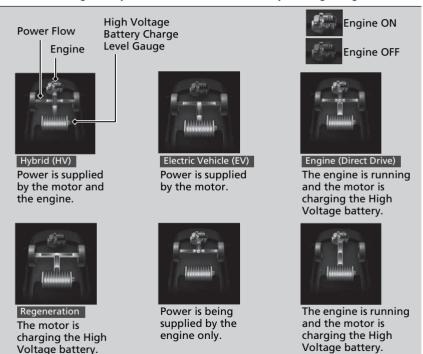
▶ Power Flow/Engine Status Display/High Voltage Battery Charge Level Gauge
