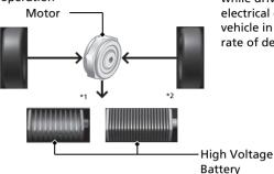
When decelerating without the accelerator being depressed or the brake pedal being applied, or while driving downhill, the electric motor acts as a generator that recovers a portion of the electrical energy that was used to accelerate the vehicle. This regenerative braking slows the vehicle in a manner similar to engine braking in a gasoline-powered vehicle. You can control the rate of deceleration by using the deceleration paddle selector.
