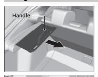
The cargo area cover can be used to cover the cargo space. ■ To pull out
