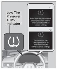
This will cause the low tire pressure/TPMS indicator to come on and a message to appear on the gauge.
