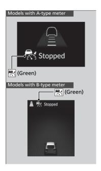
If no vehicle is ahead of you before you resume driving, depress the accelerator pedal and ACC with Low Speed Follow will operate again within the prior set speed.
