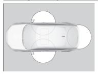
When you carry the keyless remote, you can lock/unlock the doors, fuel fill door, and hatch.
