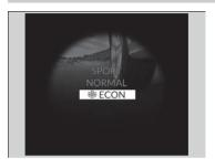
Facilitates fuel-efficient driving.
