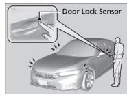
Touch the door lock sensor on the front door or press the lock button on the hatch.
