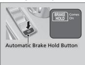
Fasten your seat belt properly, then turn the power system on. Press the automatic brake hold button.
