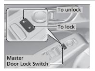
Press the master door lock switch in as shown to lock or unlock all doors, hatch, and fuel fill door.
