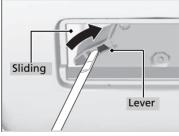
2. To open the hatch, push the hatch while sliding the lever with the flat-tip screw driver.
