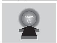
If you carry the keyless remote and press **POWER** button without depressing the brake pedal, the power mode will change in this order:
