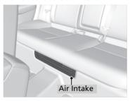
If the air intake is obstructed during vehicle operation, the High Voltage battery can become too hot. To protect the battery, the system may start to limit the battery's output and cause the power system and 12-volt battery charging system indicators to come on.
