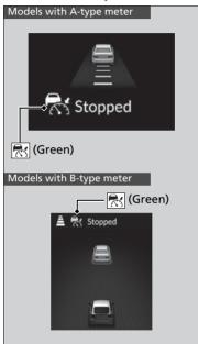
Your vehicle also stops automatically. The **Stopped** message appears on the gauge. When the vehicle ahead of you starts again, if you press the **RES/+/SET/-** switch up or down, or depress the accelerator pedal, ACC with Low Speed Follow will operate again within the previously set speed.
