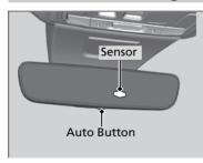
When you are driving after dark, the automatic dimming rearview mirror reduces the glare from headlights behind you. Press the AUTO button to turn this function on and off. When activated, the AUTO indicator comes on.
