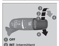
The rear wiper and washer can be used when the power mode is in ON.
