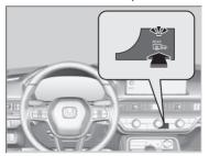
The rear defogger and heated door mirror automatically switch off after 10-30 minutes depending on the outside temperature. However, if the outside temperature is 32°F (0°C) or below, it does not automatically switch off.
