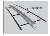
**4.** Remove the retainers from wiper blade and mount to a new rubber blade.
