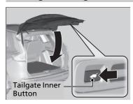
Press the tailgate inner button on the tailgate to close the power tailgate.
