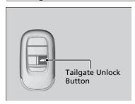
Press the tailgate unlock button to unlock the tailgate.
