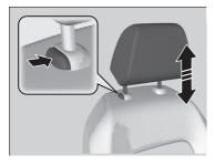
Head restraints are most effective for protection against whiplash and other rearimpact crash injuries when the center of the back of the occupant's head rests against the center of the restraint. The tops of the occupant's ears should be level with the center height of the restraint.
