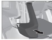
**3.** Pull the light assembly out of the rear pillar.
