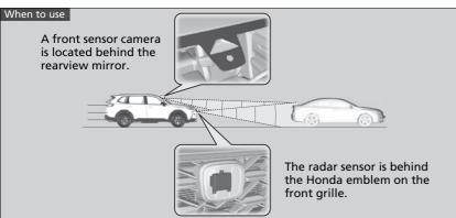
The system starts monitoring the roadway ahead when your vehicle speed is about 3 mph (5 km/h) or above and will search for a vehicle (including motorcycles), pedestrian, or moving bicycle in front of you.
