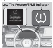
This will cause the low tire pressure/TPMS indicator to come on and a message to appear on the gauge.
