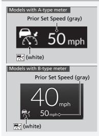
The set speed cannot be set or resumed when ACC with Low Speed Follow has been turned off using the button. Press the button to activate the system, then set the desired speed.
