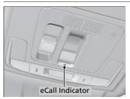
If your vehicle is involved in a collision, the vehicle will attempt to connect to an operator. Once a connection is established, your location information will be sent to an operator with whom you will be able to speak.
