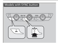
Pressing the (windshield defroster) button turns the air conditioning system on and automatically switches the system to fresh air mode.
