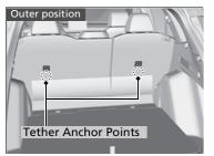
A tether anchor point is provided behind the rear outer seating positions and in the ceiling for the rear center.
