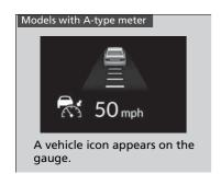
When a vehicle whose speed is slower than your set speed comes in or cuts in front of you and is detected by the radar and the camera, your vehicle starts to slow down.
