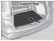
**4.** Push the far end of the floor lid down to the bottom under the support rods, then lower the other end.
