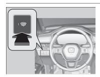
Press the heated windshield button to deice the windshield at the wiper park area and along the driver side edge of the windshield when the power mode is in ON.
