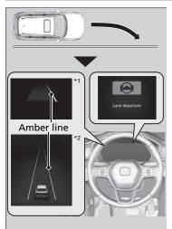
The front camera behind the rearview mirror monitors left and right lane markings in white or yellow, the outer edge of the pavement (bordered by grass or gravel road shoulder) or a detected oncoming vehicle.
