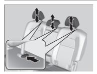
A passenger sitting in the rear seat should adjust the height of their head restraint to an appropriate position before the vehicle begins moving.
