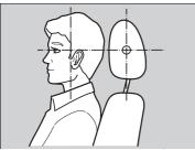
Position head in the center of the head restraint.
