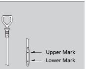
**4.** Remove the dipstick again, and check the level. It should be between the upper and lower marks. Add oil if necessary.
