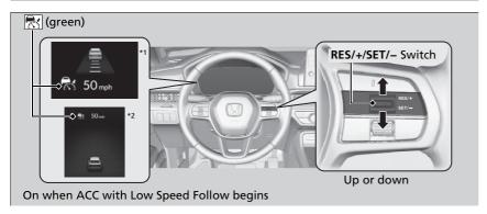
When driving at about 20 mph (30 km/h) or above: Take your foot off the pedal and press the RES/+/SET/– switch up or down when you reach the desired speed. The moment you release the switch, the set speed is fixed, and ACC with Low Speed Follow begins.
