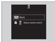
Roll the right selector wheel to scroll to select **Reduce traction control**, then press the right selector wheel to check or uncheck it.
