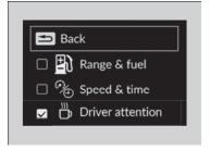
**3.** Roll the right selector wheel to scroll between contents, then press the right selector wheel to check or uncheck them.
