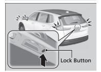
Touch the door lock sensor on the front door or press the lock button on the tailgate.
