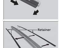
**4.** Remove the retainers from wiper blade and mount to a new rubber blade.
