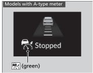
Your vehicle also stops automatically. The **Stopped** message appears on the gauge. When the vehicle ahead of you starts again, if you press the **RES/+/SET/-** switch up or down, or depress the accelerator pedal, ACC with Low Speed Follow will operate again within the previously set speed.
