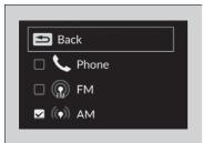
**3.** Roll the left selector wheel to scroll between audio sources, then press the left selector wheel to check or uncheck them.
