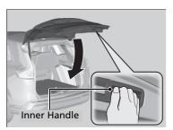
When all the doors are unlocked or you press the tailgate unlock button\* on the remote transmitter, the tailgate is unlocked. Press the tailgate outer handle and lift open the tailgate.
