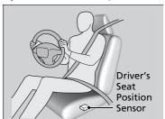
The driver's advanced airbag system includes a seat position sensor.
