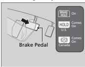
Depress the brake pedal to come to a complete stop. The transmission must not be in  $\boxed{P}$  or  $\boxed{R}$ .
