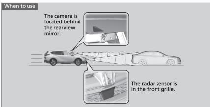
The system starts monitoring the roadway ahead when your vehicle speed is about 5 km/h (3 mph) and there is a vehicle in front of you.
