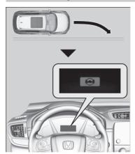
The front camera behind the rearview mirror monitors left and right lane markings (in white or yellow) and the outer edge of the pavement (bordered by grass or gravel). If your vehicle is getting too close to detected lane markings or the outer edge of the pavement (bordered by grass or gravel) without a turn signal activated, the system, in addition to a visual alert, applies steering torque and alerts you with rapid vibrations on the steering wheel, to help you remain within the detected lane.
