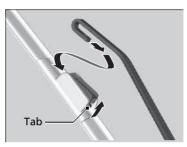
**4.** Press up on and hold the tab, then slide the holder off the wiper arm.
