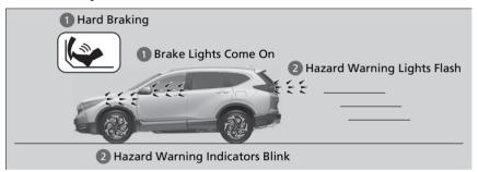
The hazard warning lights stop flashing when:
