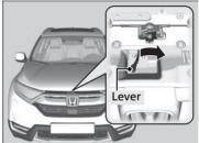
**3.** Push the bonnet latch lever (located under the front edge of the bonnet to the centre) to the side and raise the bonnet. Once you have raised the bonnet slightly, you can release the lever.
