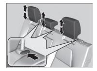
A passenger sitting in the second row seat seating position should adjust the height of their head restraint to an appropriate position before the vehicle begins moving.
