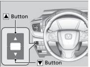
When the head-up display is on, press and hold the **HUD** button until its brightness level indicator on the driver information interface. **Brighten:** Press the ▲ button. **Dim:** Press the ▼ button.
