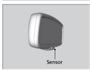
When you are driving after dark, the automatic dimming rearview mirror reduces the glare from headlights behind you, based in inputs from the mirror sensor. This feature is always active.
