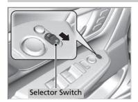
If activated, the passenger side door mirror automatically tilts downward when you put the transmission into [R]; this improves closein visibility on the passenger side of the vehicle when backing up. The mirror automatically returns to its original position when you take the transmission out of  $\mathbb{R}$ .
