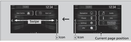
Selecting  $\langle\!\langle\!\langle|$  or  $|\!\rangle\!\rangle\!\rangle$ , or swiping the screen left or right changes to the next screen.
