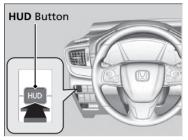
You can operate the head-up display to press the **HUD** button for about one second when the power mode is in ON.
