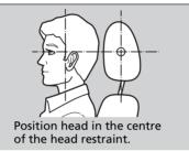
Head restraints are most effective for protection against whiplash and other rearimpact crash injuries when the centre of the back of the occupant's head rests against the centre of the restraint. The tops of the occupant's ears should be level with the centre height of the restraint.
