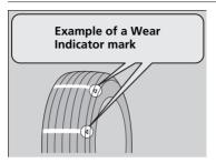
The groove where the wear indicator is located is about 1.6 mm (about 1/16 inch) shallower than elsewhere on the tyre. If the tread has worn so that the indicator is exposed, replace the tyre.
