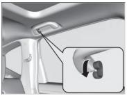
There are coat hooks on the rear left and right grab handles. Pull it down to use it.
