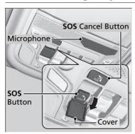
If you need to make an emergency call, you can establish a connection manually: Press the **SOS** button and hold it for more than 0.5 seconds.
