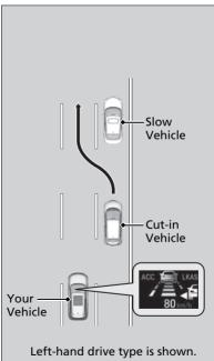
The radar sensor in the front grille detects vehicles ahead of you including those in the adjacent lane, and the camera behind the rearview mirror detects the lane markings.
