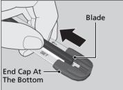
**5.** Pull the end of the wiper blade in the direction of the arrow in the image until it is out of the holder's end cap.
