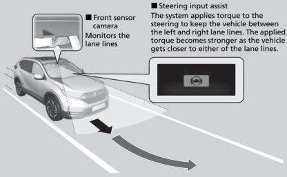
When you operate the turn signals to change lanes, the system is suspended, and resumes after the signals are off.
