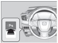
With the ignition switch is ON  $\boxed{II}^{*1}$ , press the parking sensor system button to turn on or off the system. The indicator in the button comes on when the system is on.
