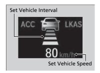
When ACC with LSF starts operating, the vehicle icon, interval bars and set speed appear on the driver information interface.
