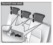
A passenger sitting in the second row and third row seating position should adjust the height of their head restraint to an appropriate position before the vehicle begins moving.
