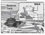
The fluid level should be between the **MIN** and **MAX** marks on the side of the reserve tank
