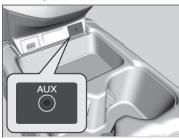
Connect a device to the input jack using a 3.5 mm stereo miniplug.
