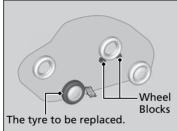
**9.** Place a wheel block or rock in front and rear of the wheel diagonal to the flat tyre.
