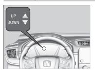
Come on to notify you that a gear change is recommended in order to maintain fuel efficient driving or to prevent the engine from stalling.
