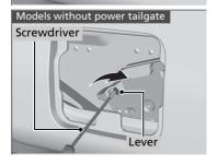
**2.** To open the tailgate, push the tailgate while pushing the lever to the right.
