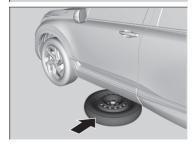
**10.** Place the compact spare tyre (wheel side up) under the vehicle body, near the tyre that needs to be replaced.
