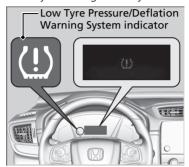
This will cause the low tyre pressure/deflation warning system indicator to come on and a message to appear on the driver information interface.
