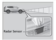
The radar sensor is in the front grille.
