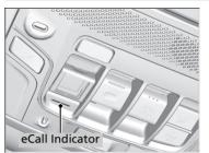
If your vehicle is involved in a collision, the SRS unit in the vehicle will attempt to connect to a Public Safety Answering Point (PSAP) operator. Once a connection is established, various information about the vehicle will be sent to a PSAP operator with whom you will be able to speak. This information includes:
