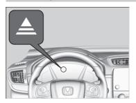
Comes on while the vehicle is in the 7-speed manual shift mode to indicate when shifting is appropriate to maintain the most fuel efficient driving style.
