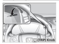
When the brightness of the meter is reduced, you can use the (TRIP) knob to adjust instrument panel brightness.
