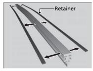
**4.** Remove the retainers from wiper blade and mount to a new rubber blade.
