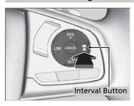
Press the (interval) button to change ACC following-interval.
