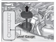
Check the amount of window washer fluid using the washer fluid level gauge on the cap.
