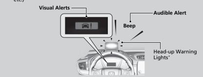
At system's earliest collision alert stage, you can change the distance (**Far/Normal/Near**) between vehicles at which alerts will come on through the driver information interface or audio/information screen setting options.
