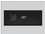
If the system operates several times without detecting driver response, the system beeps to alert you. After that, the Road Departure Mitigation steering assist is temporarily stopped, and the warning sound is given only.
