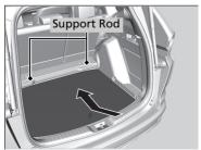
**4.** Push the far end of the floor lid down to the bottom under the support rod, then lower the other end.
