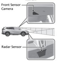
The radar sensor is in the front grille.
