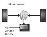
When decelerating without the accelerator being depressed or the brake pedal being applied, or while driving downhill, the electric motor acts as a generator that recovers a portion of the electrical energy that was used to accelerate the vehicle. This regenerative braking slows the vehicle in a manner similar to engine braking in a gasoline-powered vehicle. This function is enhanced when the shift lever is moved to B.
