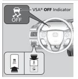
This button is on the driver side control panel. To partially turn the VSA features on and off, press and hold it until you hear a beep.
