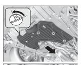
1. Remove the engine under cover.
