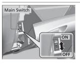
The trunk main switch disables the trunk release button on the remote transmitter and the trunk release button on the trunk lid to protect luggage in the trunk.
