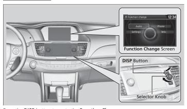
Press the **DISP** button to go to the **Function Change** screen. Rotate ? to select **Audio**, **Phone**, **Info** or **Settings** and press 8.
