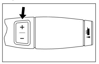
On vehicles with a Range Selection Mode. The Range Selection Mode controls the vehicle's transmission.
