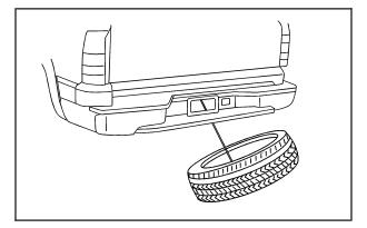
Tilt the tire toward the vehicle. Separate the tire/wheel retainer (G) from the guide pin. Pull the pin through the center of the wheel. Tilt the retainer down and through the center wheel opening.
