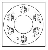
Tighten the nuts firmly in a crisscross sequence as shown by turning the wheel wrench clockwise.
