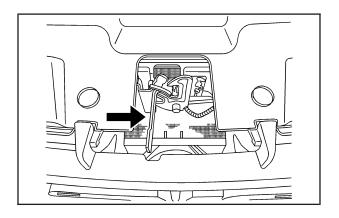
Then go to the front of the vehicle and locate the secondary hood release, near the center of the grille.
