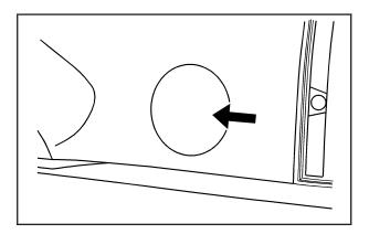
To open the fuel door, push the rearward center edge inboard and release. The door will pop open.
