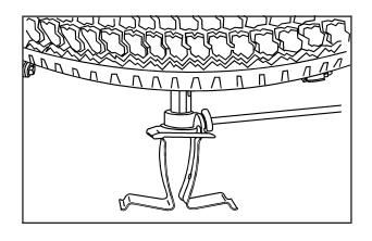
Attach the jack handle, extension, and wheel wrench to the jack and place it (with the wheel blocks) under the vehicle toward the front of the rear bumper.
