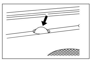
The solar sensor, located in the defrost grille in the middle of the instrument panel, monitors the solar radiation. Do not cover the solar sensor or the system will not work properly.
