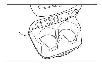
To access the cupholders in the rear floor console, pull downward on the lid.
