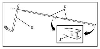
4. Assemble the two jack handle extensions (D) and wheel wrench (E) as shown.
