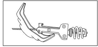
Make sure the retainer is fully seated across the underside of the wheel.
