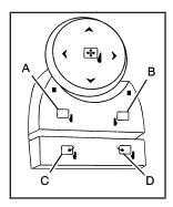
The outside power foldaway mirror controls are located on the driver's door armrest.
