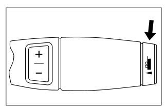
Your vehicle has a tow/haul mode. The tow/haul mode adjusts the transmission shift pattern to reduce shift cycling, providing increased performance, vehicle control, and transmission cooling when towing or hauling heavy loads.
