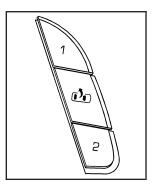
The controls for this feature are located on the driver's door panel, and are used to program and recall memory settings for the driver's seat, outside mirrors, and the adjustable throttle and brake pedal feature if your vehicle has it.
