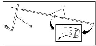
Assemble the two jack handle extensions (D) and wheel wrench (E) as shown.
