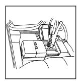
6. Connect the red positive (+) cable to the positive (+) terminal of the vehicle with the dead battery. Use a remote positive (+) terminal if the vehicle has one.
