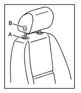
Pull the head restraint up to raise it. To lower the head restraint, press the release button (A), located on the top of the seatback, while you push the head restraint down.
