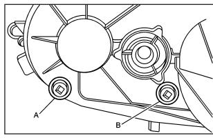
(A) Drain Plug (B) Filler Plug
