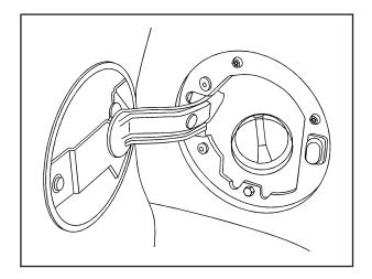
The tethered fuel cap is located behind a hinged fuel door on the driver's side of the vehicle.
