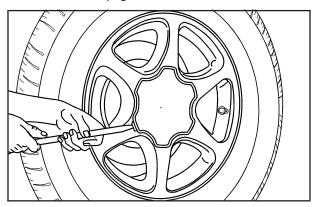
If the wheel has a center cap that covers the wheel nuts, place the chiseled end of the wheel wrench in the slot on the wheel and gently pry the cap out.
