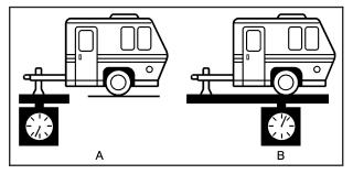
The trailer tongue weight (A) should be 10 percent to 15 percent of the total loaded trailer weight (B), up to a maximum of 600 lbs (272 kg) with a weight carrying hitch. The trailer tongue weight (A) should be 10 to 15 percent of the total loaded trailer weight, up to a maximum of 1,000 lbs (453 kg) with a weight distributing hitch.
