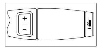
Press this button at the end of the shift lever to enable tow/haul mode.
