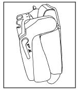
Lift the lever again to release the rear of the seat from the floor. The seat will tumble forward.
