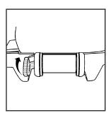
Unlatch the seat from the floor by lifting the lever located next to the carrying handle on the rear of the seat near the bottom.
