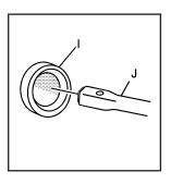
Insert the open end of the extension (J) through the hole in the rear bumper (I) (hoist shaft access hole).
