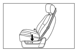
The controls used to operate the power lumbar feature are located on the outboard side of the seats.
