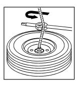
Use the wheel wrench hook that allows you to pull the hoist cable towards you, to assist in reaching the spare tire.
