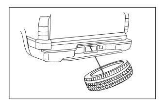
Tilt the tire toward the vehicle with some slack in the cable to access the tire/wheel retainer (G). Separate the retainer from the guide pin by sliding the retainer up the pin while pressing down on the latch.
