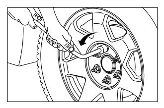
Use the wheel wrench to loosen all the wheel nuts. Turn the wheel wrench counterclockwise to loosen the wheel nuts. Do not remove the wheel nuts yet.
