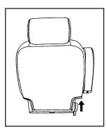
Lift the lever, located on the bottom rear of the second row seat on the inboard side, to release the seatback. The seatback will fold forward.
