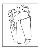
Lift the same lever again to release the rear of the seat from the floor. The seat will tumble forward.
