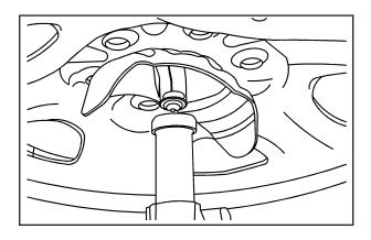
Position the center lift point of the jack under the center of the spare tire.
