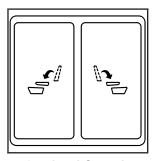
From the front seats, press one of the automatic seat release buttons located on the overhead console.
