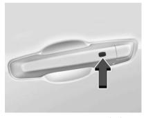
The remote key must be within 1 m (3 ft) of the liftgate or door being opened. Press the button on the front door handle to open. See *Remote Key Operation* ❖ 7.
