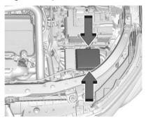
There are two clips on the side of the fuse block cover. See Engine Compartment Overview
