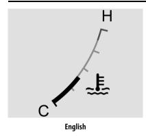
This gauge shows the engine coolant temperature.
