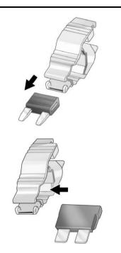
3. Use the fuse puller to remove the fuse from the top or side.
