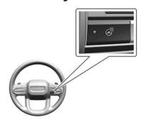
: If equipped, press to turn the heated steering wheel on or off. A light next to the button displays when the feature is turned on. The steering wheel takes about three minutes
