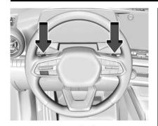
Electronic Range Select (ERS), or Manual Mode, allows for the selection of the range of gear positions. Use this mode when driving downhill or towing a trailer to limit the top gear and vehicle speed. The shift position indicator within the Driver Information Center (DIC) will display a number next to the L indicating the highest available gear.
