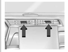
Use the air outlets in the center and on the side of the instrument panel to direct the airflow. move the center knobs on the air outlets to open or close off the airflow.
