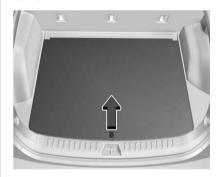
Lift the load floor to access the storage area.
