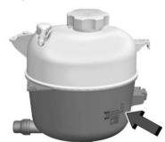
Check to see if coolant is visible in the coolant surge tank. If the coolant inside the coolant surge tank is boiling, do not do anything else until it cools down. If coolant is visible
