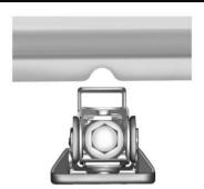
Position the jack lift head at the jack location nearest the flat tire. The location is indicated by a notch in the vertical bottom edge of the body side sheet metal.
