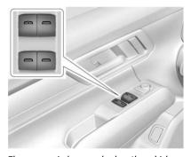
The power windows work when the vehicle is on, in accessory mode, or when Retained Accessory Power (RAP) is active. See Retained Accessory Power (RAP) ⇔ 167.
