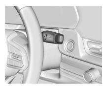
The shift pattern is displayed on the front of the shift lever. The selected gear position will illuminate red on the shift lever, while all others will be displayed in white. If the shift is not immediate, as in very cold conditions, the indicator on the shift switch may blink until it is fully engaged.
