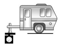
The trailer tongue weight contributes to the Gross Vehicle Weight (GVW). GVW includes the CURB WEIGHT of your vehicle, any passengers, cargo, equipment, and the trailer tongue
