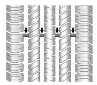
Treadwear indicators are one way to tell when it is time for new tires. Treadwear indicators appear when the tires have only 1.6 mm (1/16 in) or less of tread remaining. See *Tire Inspection* ♀ 260 and *Tire Rotation* ♀ 260.
