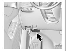
The instrument panel fuse block is under the instrument panel on the driver side.
