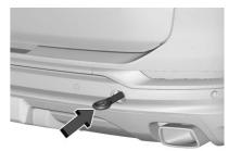
Install the tow eye into the socket and turn it until it is fully tightened.
