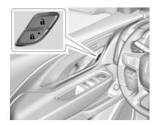
: Press to lock the doors. The indicator light in the switch will come on when the door is locked.
