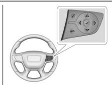
Press  $\triangleleft$  or  $\triangleright$  to select VEHICLE menu, then use  $\triangle$  or  $\nabla$  to scroll through the menu items to select TCS/StabiliTrak/ESC.
