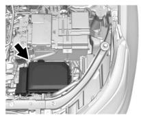
To remove the fuse block cover, squeeze the clips on the cover and lift it straight up. See Engine Compartment Overview
