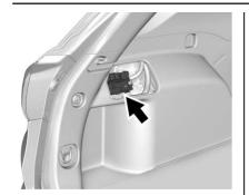
Remove the trim plate to access the fuse block.
