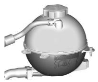
Check to see if coolant is visible in the coolant surge tank. If the coolant inside the coolant surge tank is boiling, do not do anything else until it cools down. If coolant is visible but the coolant level mark is not visible, add a 50/50 mixture of clean, drinkable water and DEX-COOL coolant at the coolant surge tank to the top rib on the middle of the tank, but be sure the cooling system is cool before this is done. See Engine Overheating \$\triangle\$ 270.
