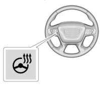
: If equipped, press to turn it on or off. A light next to the button displays when the feature is turned on.
