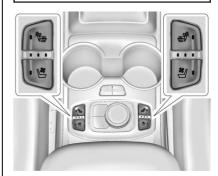
If equipped, the buttons are on the center console. To operate, the engine must be running.
