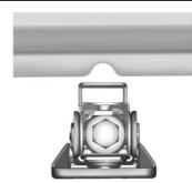
Position the jack lift head at the jack location nearest the flat tire. The location is indicated by a notch in the vertical bottom edge of the body side sheet metal.
