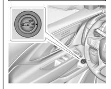
The power liftgate switch is on the driver door. The vehicle must be in P (Park). The taillamps flash when the power liftgate moves.
