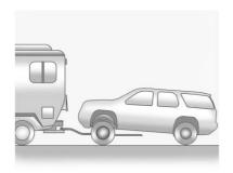
Tow the vehicle with the two rear wheels on the ground and the front wheels on a dolly.
