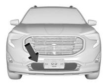
Center grille cover and make sure that it is positioned correctly.
