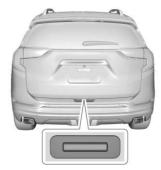
To open the liftgate, press on the power door lock switch or press on the RKE transmitter twice to unlock all doors. Press the touch pad on the underside of the liftgate handle and lift up.
