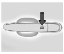
The RKE transmitter must be within 1 m (3 ft) of the liftgate or door being opened. Press the button on the door handle to open. See "Keyless Access Operation" in Remote Keyless Entry (RKE) System Operation
