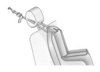
If the position you are using has an adjustable headrest or head restraint and you are using a dual tether, raise the headrest or head restraint and route the tether under the headrest or head restraint and in between the headrest or head restraint posts.
