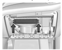
Remove the two screws securing the door.
