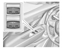
The power windows work when the ignition is on, in ACC/ACCESSORY, or in Retained Accessory Power (RAP). See Retained Accessory Power (RAP) ⇒ 204.
