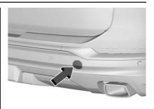
If equipped, carefully open the cover by using the small notch that conceals the rear tow eye socket.
