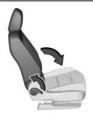
Lift the lever fully and fold the seatback forward.
