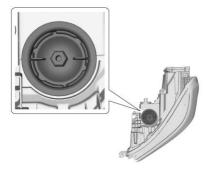
Remove the bulb access cap from the top of the headlamp assembly by turning it counterclockwise.
