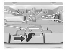
Go to the front of the vehicle and locate the secondary release lever under the front center of the hood. Push the secondary hood release lever to the right to release.
