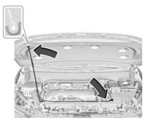
Lift the hood and release the hood prop rod from its retainer in the front of the engine compartment. Securely insert the rod end into the slot marked with an arrow, on the underside of the hood.
