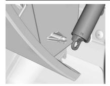
Disconnect the glove box door damper (1) from the glove box door assembly by squeezing the pivot (2) to release the damper ring.
