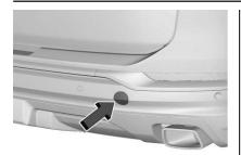
If equipped, carefully open the cover by using the small notch that conceals the rear tow eye socket.
