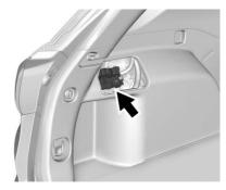
Remove the trim plate to access the fuse block.
