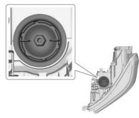
Remove the bulb access cap from the top of the headlamp assembly by turning it counterclockwise.
