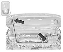
Release the hood prop from its retainer, located above the radiator. Securely place the hood prop into the slot on the underside of the hood.
