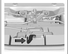
Go to the front of the vehicle to find the secondary hood release handle. The handle is under the front edge of the hood near the center. Push the handle to the right and raise the hood.
