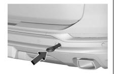
Install the tow eye into the socket by turning it until it stops.
