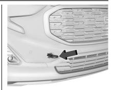
Install the tow eye into the socket by turning it until it stops.
