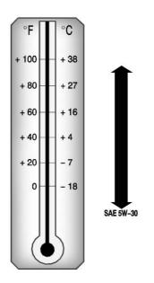
Cold Temperature Operation: In an area of extreme cold, where the temperature falls below -29 °C (-20 °F), an SAE 0W-40 oil may be used. An oil of this viscosity grade
