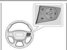
Press  $\triangleleft$  or  $\triangleright$  to select VEHICLE menu, then use  $\triangle$  or  $\nabla$  to scroll through the menu items to select TCS/StabiliTrak/ESC.
