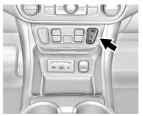
ERS or manual mode allows for the selection of the range of gear positions. Use this mode when driving downhill or towing a trailer to limit the top gear and vehicle speed. The shift position indicator within the Driver Information Center (DIC) will display a number next to the L indicating the highest available gear under manual mode and the driving conditions when manual mode was selected.
