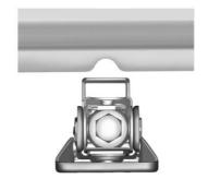
Locate the notch on the sheet metal weld flange. Place the center of the jack lift head on the center of the sheet metal notch.
