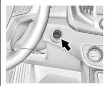
The vehicle has an electronic keyless ignition with pushbutton start.
