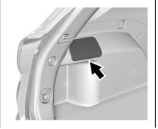
The rear compartment fuse block is behind a trim panel on the side of the rear compartment.
