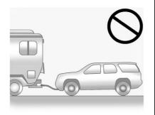
The vehicle was not designed to be towed with all four wheels on the ground. The vehicle may be towed using a platform trailer with all four wheels off the ground. Some vehicles may be dolly towed. See the following information on dolly towing.
