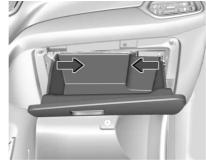
Squeeze both sides of the glove box bin inward to lower beyond the stops.
