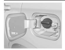
The fuel cap is behind a hinged fuel door on the driver side of the vehicle. To open the fuel door, push and release the rearward center edge of the door.
