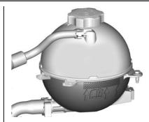
Check to see if coolant is visible in the coolant surge tank. If the coolant inside the coolant surge tank is boiling, do not do anything else until it cools down. If coolant is visible but the coolant level mark is not visible, add a 50/50 mixture of clean, drinkable water and DEX-COOL coolant at the coolant surge tank to the top rib on the middle of the tank, but be sure the cooling system is cool before this is done. See *Engine Overheating* \$\psi\$ 305.
