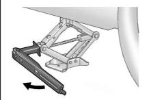
Raise the vehicle by turning the wheel wrench clockwise. Raise the vehicle far enough off the ground so there is enough room for the road tire to clear the ground.
