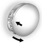
The fuel cap is behind the fuel door on the passenger side of the vehicle. To open the fuel door, push and release the rearward center edge of the door.
