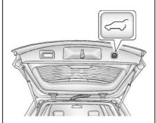
Press and release  $\leftarrow$  on the liftgate next to the latch to close the liftgate.
