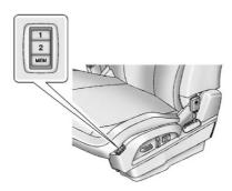
If available, the 1, 2, and MEM (Memory) buttons on the outboard side of the driver seat are used to manually save and recall the driver seat and outside mirror positions. These manually stored positions are referred to as Button Memory positions.
