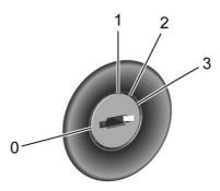
The ignition switch has four different positions.
