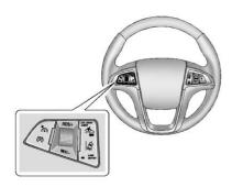
To turn LDW on and off, press the LANE DEPART button on the steering wheel. The control indicator will light when LDW is on.
