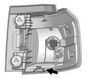
Verify that the taillamp assembly tab, located at the bottom of the taillamp assembly, is aligned to the fascia bracket before securing with screws.
