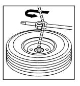
Use the wheel wrench which has a hook that allows you to pull the hoist cable towards you to assist in reaching the spare tire.
