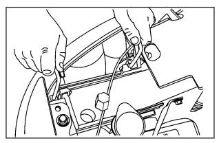
Remove the two pins on the top of the headlamp assembly. To remove the outer pin, turn outward and pull it straight up. To remove the inner pin, turn it in and pull it straight up.
