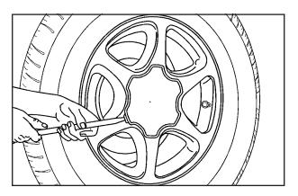
Remove the center cap by placing the chisel end of the wheel wrench in the slot on the wheel and gently prying the cap out.
