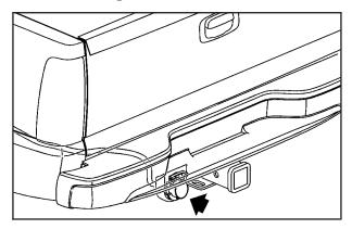
Your pickup is equipped with the eight-wire trailer towing harness. This harness with a seven-pin universal heavy-duty trailer connector is attached to a bracket on the hitch platform.
