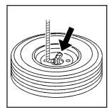
Tilt the retainer downward and through the wheel opening.
