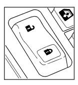
If your vehicle is equipped with power door locks, press the raised side of the switch, with the lock symbol, on either front door to lock all the doors at once.
