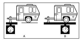
The trailer tongue weight (A) should be 10 percent to 15 percent of the total loaded trailer weight (B), up to a maximum or 600 lbs (272 kg) with a weight carrying hitch. The trailer tongue weight (A) should be 10 percent to 15 percent of the total loaded trailer weight, up to a maximum of 1,000 lbs (453 kg) with a weight distributing hitch.
