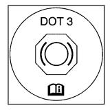
Your brake master cylinder reservoir is filled with DOT-3 brake fluid. See *Engine Compartment Overview on page 5-10* for the location of the reservoir.
