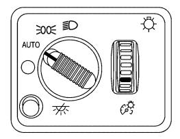
The control on the driver's side of the instrument panel operates the exterior lamps.
