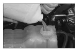
Fill the coolant surge tank with the proper mixture, to the FULL COLD mark.
