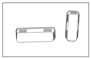
**Vertical Control:** You can use the vertical control of the power seat controls to adjust the angle of the seatback. Press the control rearward to recline the seatback. Press the control forward to raise the seatback.
