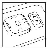
If your vehicle is equipped with this feature, the controls are located on the driver's door armrest.
