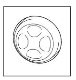
You can increase or decrease lumbar support in an area of the lower seatback with this control, located on the outboard sides of the front seat(s).
