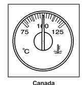
This gage shows the engine coolant temperature.
