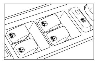
A power window control is located on the inside of each door.
