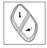
**7:** (Trip Information): Press this button to display the odometer, trip odometers, timer, and engine hours.
