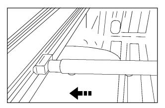
Remove the two bows by gently pushing them against the spring-loaded end. The two bows are labeled front and rear to remind you of the order in which to reinstall them.
