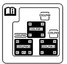
The auxiliary electric cooling fan fuse block is located in the engine compartment on the driver's side of the vehicle next to the underhood fuse block.
