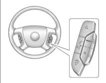
△ or ➢ / ▽: Press to change favorite radio stations, select tracks on a CD/DVD, or navigate tracks or folders on an iPod® or USB device.
