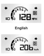
Format Three: This display includes all the information in Format One along with a circular tachometer, but without outside air temperature.
