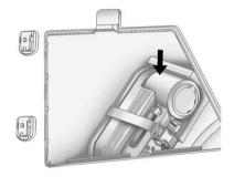
Press down on the latch tab and pull the cover off to access the storage compartment.
