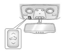
The switch to operate the front sunroof is on the headliner above the rearview mirror.
