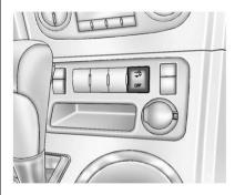
To change the liftgate to manual operation, press OFF on the power liftgate switch. A message displays on the DIC indicating manual operation mode. See Driver Information Center (DIC) (Without DIC Buttons) on page 5-30 or Driver Information Center (DIC) (With DIC Buttons) on page 5-25.
