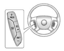
The cruise control buttons are located on left side of the steering wheel.
