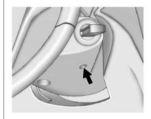
Vehicles with an automatic transmission are equipped with an electronic key lock release system. This system is to prevent ignition key removal unless the shift lever is in P (Park).
