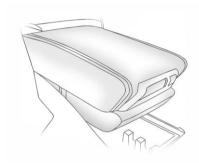
Pull up on the lever, located on the front of the center console armrest, to slide it forward and backward. To open the armrest storage area, press the button located on the front of the armrest.
