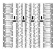
Treadwear indicators are one way to tell when it is time for new tires. Treadwear indicators appear when the tires have only 1.6 mm (1/16 in) or less of tread remaining. See *Tire Inspection on page 10-50* and *Tire Rotation on page 10-50* for more information
