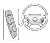
ress to turn cruise control on and off. The indicator comes on when cruise control is on.
