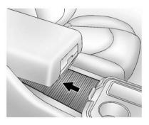
There is additional storage under the armrest. Move the armrest all the way to the rear position, then slide the storage cover back to access.
