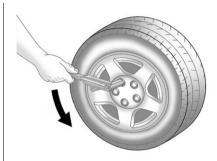
Loosen the wheel nuts — but do not remove them — using the wrench. For wheels with a wheel lock key, use the wheel lock key between the lock nut and wrench. The key is supplied in the front passenger door pocket. Notice: If this vehicle has wheel locks and an impact wrench is used to remove the wheel nuts, the lock nut or wheel lock key could be damaged. Do not use an impact wrench to remove the wheel nuts if this vehicle has wheel locks.
