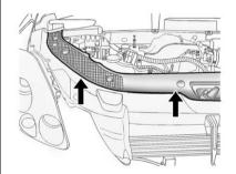
Detach the fasteners and lift off the panel that covers the radiator cap.
