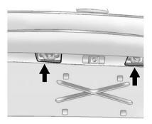
Turn and pull the license plate lamp forward through the liftgate trim opening.
