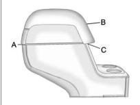
To access the upper storage area, press the upper button (B) and lift up. To access the lower storage area, press the lower button (C) and lift up. The top of the console can be folded forward for increased storage area. Lift up on the handle on the rear of the console (A) and pull forward.
