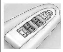
Press the switch to lower the window. Pull the switch up to raise it.
