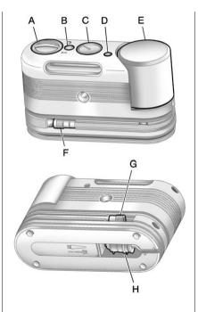
When using the tire sealant and compressor kit during cold temperatures, warm the kit in a heated environment for five minutes. This will help to inflate the tire faster.
