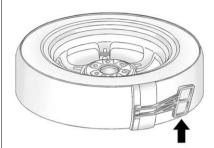
Remove the plastic spare tire heat shield by pulling the rubber latch. Store the plastic spare tire heat shield. See "Storing the Spare Tire" later in this section for more information.
