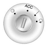
The ignition switch has four different positions.
