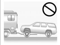
All-wheel-drive vehicles must not be towed with two wheels on the ground. To properly tow these vehicles, they should be placed on a platform trailer with all four wheels off of the ground or dinghy towed from the front.
