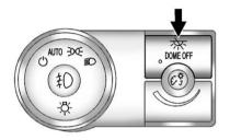
The dome lamp override button is next to the exterior lamps control.
