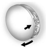
To remove the fuel cap, turn it slowly counterclockwise. The fuel cap has a spring in it; if the cap is released too soon, it will spring back to the right.
