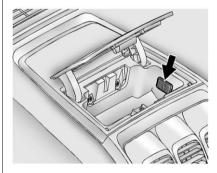
To connect a USB storage device, connect the device to the USB port located in the instrument panel storage area. See *Instrument Panel Storage on page 4-1* for more information.
