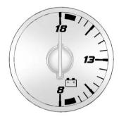
When the engine is not running, but the ignition is turned on, this gauge shows the battery's state of charge in DC volts.
