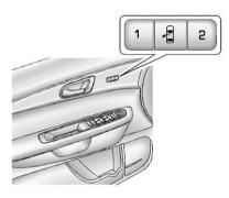
On vehicles with the memory feature, the controls on the driver door are used to program and recall memory settings for the driver seat and outside mirrors.
