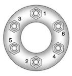
14. Tighten the wheel nuts firmly in a crisscross sequence, as shown.
