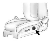
If available, press and hold the front or rear of control to increase or decrease lumbar support. Release the control when the seatback reaches the desired level of lumbar support.
