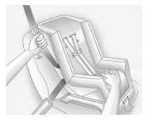
6. To tighten the belt, push down on the child restraint, pull the shoulder portion of the belt to tighten the lap portion of the belt, and feed the shoulder belt back into the retractor. When installing a forward-facing child restraint, it may be helpful to use your knee to push down on the child restraint as you tighten the belt.
