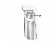
To move it down, push down on the release button (A) and move the height adjuster to the desired position. You can move the height adjuster up by pushing up on the shoulder belt guide.
