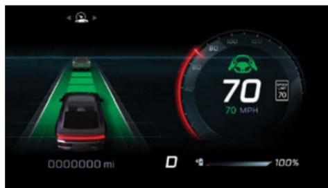
**Active Driving Assist Engaged (Steering Wheel Green)**
