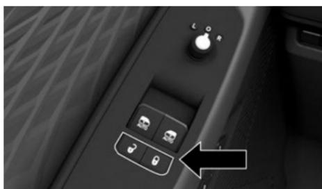
**Power Door Lock Switches (2 Door Model Shown)**
