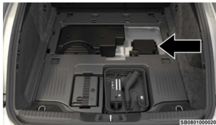
Rear Power Distribution Center
