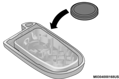
Key Fob Battery Replacement
