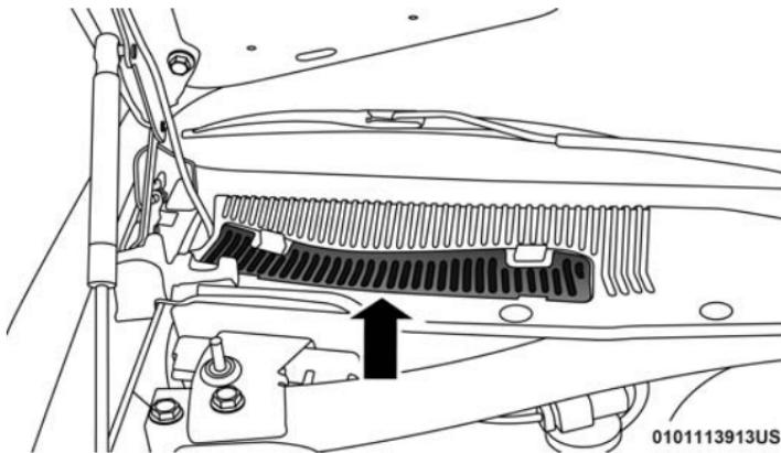
2. Unsnap both ends and lift the filter access cover.
