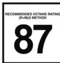
This engine is designed to meet all emissions regulations and provide excellent fuel economy and performance when using high-quality unleaded "Regular" gasoline having an octane rating of 87 as specified by the (R+M)/2 method. The use of higher octane "Premium" gasoline will not provide any benefit over "Regular" gasoline in these engines.
