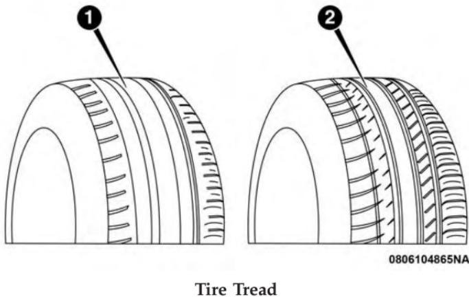
These indicators are molded into the bottom of the tread grooves. They will appear as bands when the tread depth becomes a  $1/16$  of an inch (1.6 mm).
