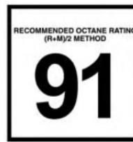
This engine is designed to meet all emission regulations, provide optimal fuel economy and performance when using high-quality unleaded "Premium" gasoline having a posted octane number of 91 as specified by the (R+M)/2 method. The use of 91 or higher octane "Premium" gasoline is required for in this engine.
