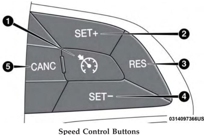
**NOTE:** In order to ensure proper operation, the Speed Control System has been designed to shut down if multiple Speed Control functions are operated at the same time. If this occurs, the Speed Control System can be reactivated by pushing the Speed Control on/off button and resetting the desired vehicle set speed.
