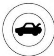
The trunk can be opened from inside the vehicle using the power trunk release button located on the instrument panel to the left of the steering wheel.
