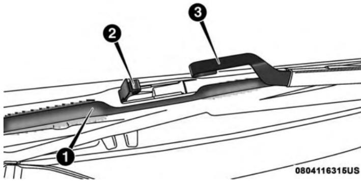
Removing Wiper From Wiper Arm
