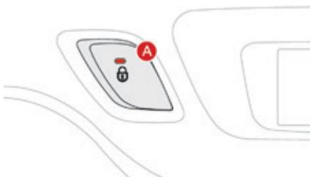
System which provides full manual locking or unlocking of the doors from the inside.
