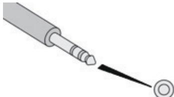
Connect the portable device (MP3 player, ...) to the auxiliary Jack socket using an audio cable (not supplied).
