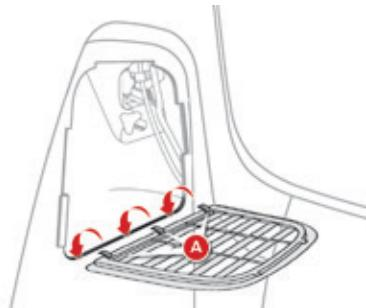
Position the three hooks **A** of the flap at the bottom.
