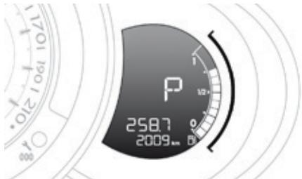
When you move the selector in the gate to select a position, the corresponding indicator is displayed in the instrument panel.
