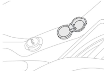
☞ To connect a 12 V accessory (max power: 120 W), lift the cover and connect a suitable adaptor.
