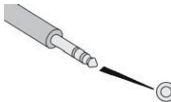
Connect the portable device (MP3 player...) to the auxiliary Jack socket using an audio cable (not supplied).
