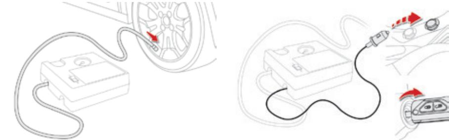
You can also use the compressor, without injecting sealant, to check and if necessary adjust the tyre pressures
