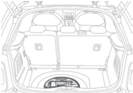
The tools are installed in the boot under the floor.
