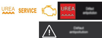
The UREA, SERVICE and diagnostic warning lamps come on, accompanied by an audible signal and the display of the message "Emissions fault".
