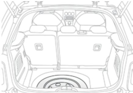
The spare wheel is installed in the boot under the floor.
