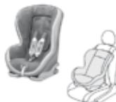
Installed only in the forward facing position.
