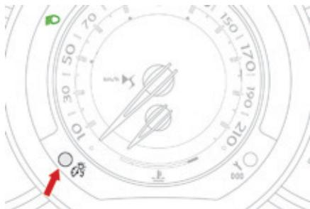
System for manual adjustment of the brightness of the instruments and controls to suit the ambient light level.
