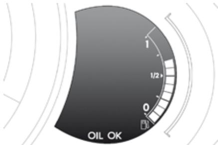
On vehicles fitted with an electric oil level indicator, information on the oil level is displayed in the instrument panel for a few seconds when the ignition is switched on, after the service information.
