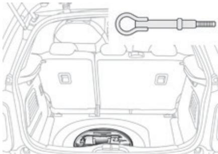
The towing eye is installed in the boot under the floor.
