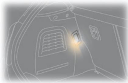
This comes on automatically when the boot is opened and goes off automatically when the boot is closed.
