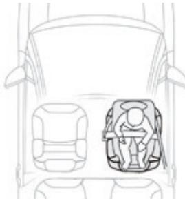
When a rearward facing child seat is installed on the **front passenger seat**, adjust the seat to the intermediate longitudinal and highest position, with the backrest straightened. The passenger's front airbag must be deactivated. Otherwise, **the child risks being seriously injured or killed if the airbag were to inflate.**
