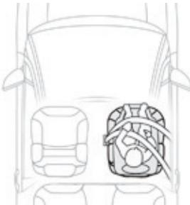
When a forward facing child seat is installed on the **front passenger seat**, adjust the vehicle's seat to the intermediate longitudinal and highest position with seat backrest straightened and leave the passenger's front airbag activated.
