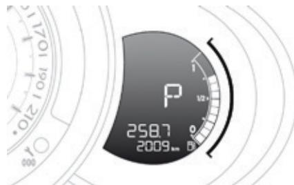
When you move the selector to select a position, the corresponding indicator is displayed in the instrument panel.
