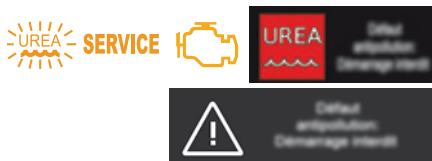
Every time the ignition is switched on, the SERVICE and engine diagnostic warning lamps come on and the UREA warning lamp flashes, accompanied by an audible signal and the display of the message "Emissions fault: Starting prevented".
