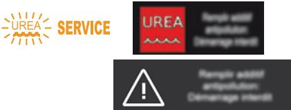
When switching on the ignition, the SERVICE warning lamp comes on and the UREA warning lamp flashes, accompanied by an audible signal and the display of the message "Top up emissions additive: Starting prevented". The AdBlue® tank is empty: the system required by regulations prevents engine starting.
