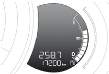
System which informs the driver when the next service is due, in accordance with the manufacturer's servicing schedule.
