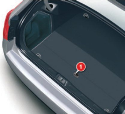
1. Boot floor (spare wheel storage).
