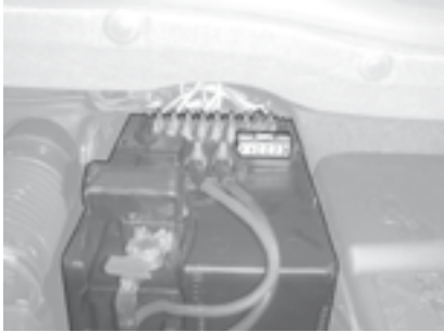
Fuses on the battery
