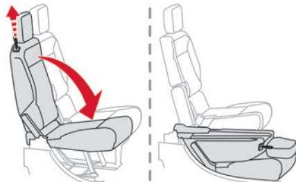
► Pull the tongue on the top edge of the seat near the head restraint to tilt and guide the assembly.
