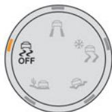
In exceptional conditions (moving a vehicle that is bogged down in mud, stuck in snow, on loose soil, etc.), it may prove useful to deactivate the
