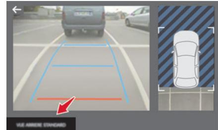
To activate the camera located on the tailgate, engage reverse gear and do not exceed a speed of 6 mph (10 km/h).
