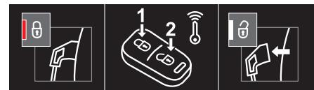
Before disconnecting the nozzle from the charging connector:
