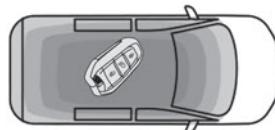
► Place the remote control inside the vehicle, in the recognition zone.
