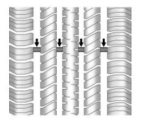
Treadwear indicators are one way to tell when it is time for new tires. Treadwear indicators appear when the tires have only 1.6 mm (1/16 in) or less of tread remaining. See *Tire Inspection* ♀ 352 and *Tire Rotation* ♀ 353.
