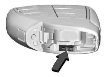
Use the mechanical key blade in the slot to remove the battery cover by hand.
