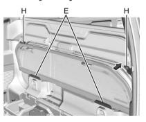
Open Corner Secures (H). Load the rear glass into the storage pocket in the midgate, guiding the lower edge of the rear glass behind the two rear glass retaining tabs (E).
