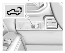
• Press on the instrument panel to the left of the steering wheel.
