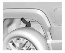
Reach around the tire to find the emergency manual charge cord release.
