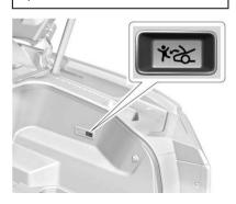
The underhood compartment is equipped with a glow-in-the-dark emergency hood release button. This button will glow following exposure to light. Press the button to open the hood from inside the underhood compartment.
