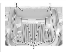
There are four hooks (1) for use with the convenience net, if equipped. The maximum load per hook is 30 kg (66 lbs).
