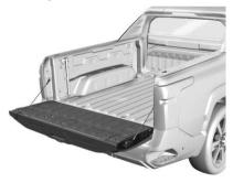
Press <sup>→</sup><sub>x2</sub> twice quickly on the remote key until the tailgate moves. See *Remote Key Operation* → 9. The tailgate can be opened if the remote key is within 1 m (3 ft).
