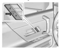
The indicator light on the driver door switch indicates the status of the system. See *Power Door Locks* ♀ 17.
