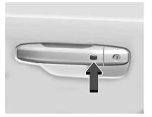
The remote key must be within 1 m (3 ft) of the eTrunk or door being opened or locked. Press the button on the door handle to open. See "Keyless Access Operation" in Remote Key Operation ♀ 9.
