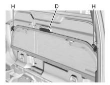
Push the glass against the glass stow retainer (D), located on the interior side of the door. Push until the glass handle slides down to lock the glass in place. Close Corner Secures (H).
