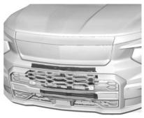
The vehicle may have a shutter system that automatically closes the frontal cooling openings. This system promotes airflow around the vehicle, reducing drag and providing energy savings. Ensure the shutter system is clear of any visible debris, snow, or ice. If the Service Vehicle Soon light activates and remains after clearing the shutter system, see Service Vehicle Soon Light (Propulsion System Failure) ⇒ 117.
