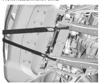
The vehicle is equipped with specific attachment points to be used to pull the vehicle onto a flatbed car carrier from a flat road surface. Do not use these attachment points to pull the vehicle from snow, mud, sand, or a ditch.
