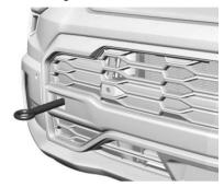
If the vehicle is equipped with a tow eye, only use the tow eye to pull the vehicle onto a flatbed car carrier from a flat road surface. Do not use the tow eye to pull the vehicle from snow, mud, sand, or a ditch.
