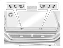
To operate, select the heated and ventilated seats launch icon. The panel will remain open for approximately five seconds.
