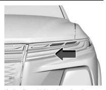
The headlamp CSI bar is located on the headlamps. As charging occurs, the blue light bars on the headlamps fill towards the center of the vehicle.
