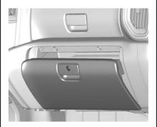
Open the lower glove box door completely.
