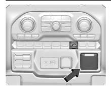
In Cab Power Outlet and DC/AC Switch
