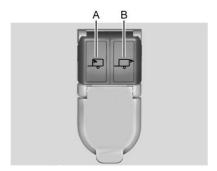
If equipped with the fifth wheel/ gooseneck trailer package, the harness connector is mounted on the inside of the pickup bed behind the rear wheel.
