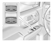
The power windows work when the ignition is on, in ACC/ACCESSORY, or when Retained Accessory Power (RAP) is active. See Retained Accessory Power (RAP) ⇒ 213.
