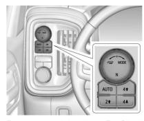
To activate and deactivate Tow/Haul turn the Drive Mode knob to the left. For activation of modes other than Tow/Haul, turn the Drive Mode knob to the right.
