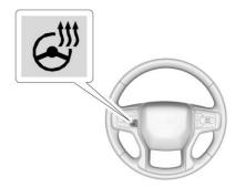
If equipped, press to turn it on or off. A light next to the button displays when the feature is turned on.
