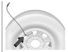
If equipped with a spare tire cable remove the cable from the spare tire by passing the clip through the looped end of the cable.
