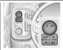
If equipped, select Terrain Mode by pressing the below the 4 ↑ transfer case button.
