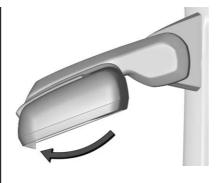
**Manual Extend**: If equipped, grasp the mirror housing firmly and pull back in one motion, arching slightly toward the rear of the vehicle.
