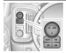
Vehicles with the MODE graphic on the knob will have a menu selection screen in the instrument cluster to select the desired mode. When the Drive Mode knob is turned to the right, the mode list will display and activate the next available mode.
