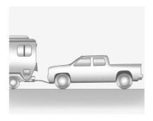
Only dinghy tow four-wheel-drive vehicles with a two-speed transfer case that have an N (Neutral) and a 4 \(\psi\) (Four-Wheel Drive Low) setting.
