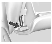
Push the dampener arm to the left until it releases the glovebox.
