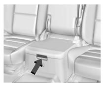
If equipped with front center seat storage, unlock with the ignition key, press the latch, and lift to open.
