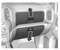
To access the upper glove box, pull up on the handle.
