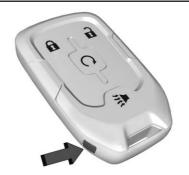
If the vehicle has the Keyless Access system, the transmitter has a button on the side of the transmitter used to remove the key.
