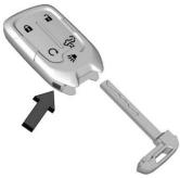
1 Press the button on the RKF transmitter to remove the key. Never pull the key out without pressing the button.
