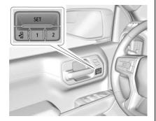
If equipped, memory seats allow two drivers to save and recall their unique seat positions for driving the vehicle, and a shared exit position for getting out of the vehicle. Other feature positions may also be saved, such as power mirrors, if equipped. Memory positions are linked to RKE transmitter 1 or 2 for automatic memory recalls.
