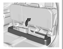
There may be storage under the rear passenger seat. Lift up on the seat bench to access. Push the seat bench toward the floor to close.
