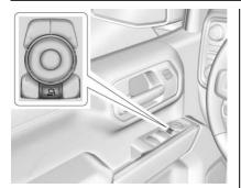
**Power Extend :** If equipped, press the power extend button to fully extend the mirror. Press again to retract.
