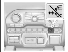
The power assist steps can be extended to the tire by pressing When extending the steps with the kick switch is disabled. The vehicle must be in P (Park) or N (Neutral).
