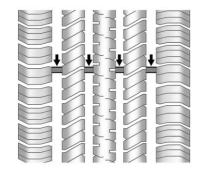
Treadwear indicators are one way to tell when it is time for new tires. Treadwear indicators appear when the tires have only 1.6 mm (1/16 in) or less of tread remaining. Some commercial truck tires may not have treadwear indicators. See *Tire Inspection* ♀ 392 and *Tire Rotation* ♀ 392 for additional information.
