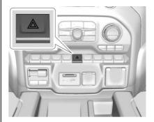
: Press this button to make the front and rear turn signal lamps flash on and off. Press again to turn the flashers off.
