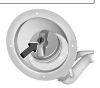
Use the fuel cap key to unlock the fuel cap then turn the fuel cap counterclockwise to remove. Fully insert and latch the fill nozzle, begin fueling.
