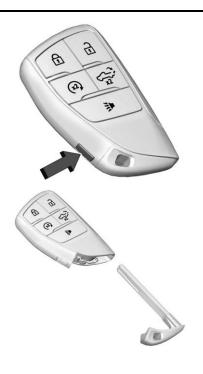
Press the button on the side of the remote key near the bottom and pull the mechanical key out. Never pull the mechanical key out without pressing the button.
