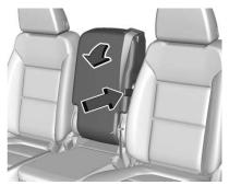
Pull the strap on the side of the center seatback to fold the center seatback. Do not use the center seatback as a seating position when the seatback is folded down.
