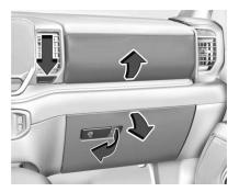
To open the upper glove box, push the button below the air outlet, to the left of the glove box.
