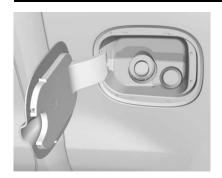
The capless refueling system does not have a fuel cap.
