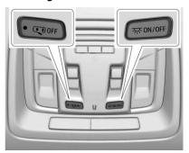
The dome light controls are in the overhead console.
