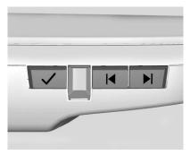
Press  $\checkmark$  to scroll through the adjustment options.
