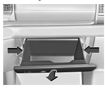
3. Press the sides of the glove box door inward and rotate the door downward to remove.
