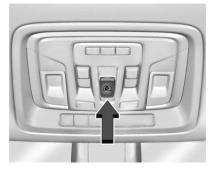
If equipped, the power sliding rear window works when the vehicle is on, in accessory mode, or Retained Accessory Power is active. See Retained Accessory Power (RAP) ⇒ 216. Press the switch to open the window and pull to close
