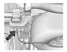
If equipped with a spare tire cable, reattach the clip to the frame attachment bracket. Note that there may be slack in the cable.
