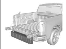
To close the inner tailgate with the primary tailgate closed, firmly push or pull it upward until it latches. Pull it back to be sure it is latched securely.
