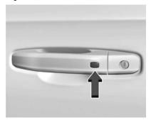
If equipped, the remote key must be within 1 m (3 ft) of the tailgate or door being unlocked or locked. Press the button on the door handle to unlock or lock. See "Keyless Access Operation" in Remote Key Operation
