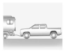
Only dinghy tow four-wheel-drive vehicles with a two-speed transfer case that have an N (Neutral) and a 4 ↓ (Four-Wheel Drive Low) setting.
