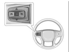
Press to turn cruise control on or off. A white indicator light comes on in the instrument cluster when cruise control is turned on. See Cruise Control Light
