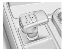
The shift pattern is displayed on the top of the shift lever. The selected gear position illuminates red on the shift lever, while all others will be displayed in white. If the shift is not immediate, as in very cold conditions, the indicator on the shift switch may blink until it is fully engaged.
