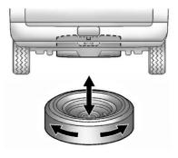
Make sure the tire is stored securely. Push, pull, and then try to turn the tire. If the tire moves, use the wheel wrench to tighten the cable.
