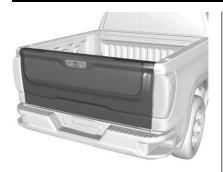
Switches in the inner tailgate prevent the primary tailgate from being opened when the inner tailgate is not fully closed.
