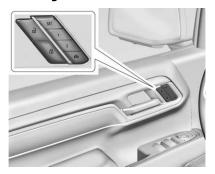
If equipped, the memory seat feature allows drivers to save their unique driving positions and a shared exit position. Other feature positions, such as power mirrors, may also be saved.
