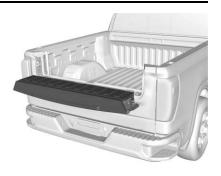
To open the inner tailgate, press the upper touch pad on the tailgate handle after unlocking all doors. Pull the top of the tailgate to open.
