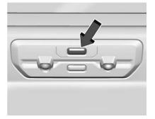
The MultiFlex inner tailgate may be equipped with an enable/disable feature to prevent the inner tailgate from being opened when a hitch or other equipment is installed that could damage the inner tailgate.
