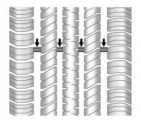
Treadwear indicators are one way to tell when it is time for new tires. Treadwear indicators appear when the tires have only 1.6 mm (1/16 in) or less of tread remaining. See *Tire Inspection* ♀ 353 and *Tire Rotation* ♀ 354.
