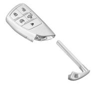
Remove the key by pressing the button on the side of the remote key near the bottom and pull the key out. Never pull the key out without pressing the button.
