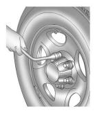
If the vehicle has wheel nut caps, loosen them by turning the wheel wrench counterclockwise.
