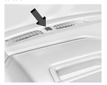
The solar sensor, on top of the instrument panel near the windshield, monitors the solar heat.
