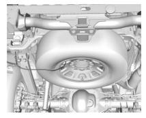
If equipped with a spare tire cable, orient the cable by rotating the spare tire so that the cable is by the frame attachment location. Raise the tire fully against the underside
