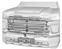
This vehicle may have a shutter system that automatically closes the frontal cooling opening. This system is designed to help improve fuel economy. If the shutter system is blocked, the Malfunction Indicator Light may turn on. Ensure the shutter system is clear of any visible debris, snow, or ice. If the Malfunction Indicator Light stays on after cleaning the shutter system, see Malfunction Indicator Light (Check Engine Light) ▷ 119.
