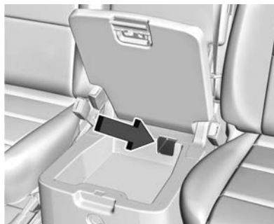
Transmitter Pocket without Bucket Seats (Lower Compartment)
