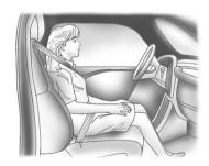
If a person of adult size is sitting in the front outboard passenger seat, but the off indicator is lit, it could be because that person is not sitting properly in the seat or that the child restraint locking feature is engaged. If this happens, use the following steps to allow the system to detect that person and enable the front outboard passenger frontal airbag:
