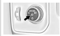
If equipped, the control is on the center of the exterior lamp control, to the left of the steering column.
