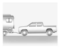
Only dinghy tow four-wheel-drive vehicles with a two-speed transfer case that have an N (Neutral) and a Four-Wheel Drive Low (4 (\dagger)) setting.
