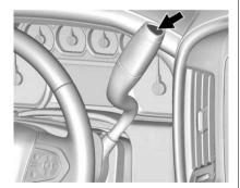
Vehicles with an automatic transmission have a Tow/Haul Mode. The Tow/Haul Mode adjusts the transmission shift pattern to reduce shift cycling. This provides increased performance, vehicle control, and enhanced transmission. and engine cooling when driving down steep hills or mountain grades, towing, or hauling heavy loads
