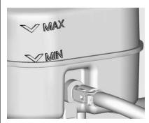
The fluid level should be above MIN. If it is not, have the brake hydraulic system checked to see if there is a leak.
