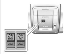
If equipped, the sunroof only operates when the ignition is in ACC/ACCESSORY or ON/RUN, or when Retained Accessory Power (RAP) is active. See Retained Accessory Power (RAP) on page 9-28.
