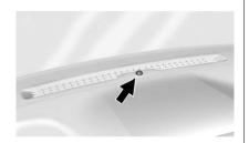
If equipped with the anti-theft alarm system, the indicator light, on the instrument panel near the windshield, indicates the status of the system.
