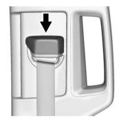
Push down on the release button to move the height adjuster to the desired position.
