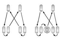
Use this rotation pattern when rotating the tires if the vehicle has dual rear wheels (except polished forged aluminum wheels).
