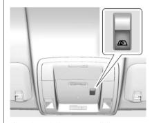
If equipped, the power sliding rear window works when the ignition has been turned to ACC/ACCESSORY or ON/RUN, or when Retained Accessory Power (RAP) is active. See Retained Accessory Power (RAP) on page 9-28.
