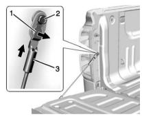
Raise the tailgate and support it firmly. Pull out and hold the cable retaining clip (1). Push the cable (3) up and off of the bolt (2). Repeat on the other side.
