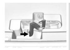
Go to the front of the vehicle to find the secondary hood release. The handle is under the front edge of the hood near the center. Push the handle to the right and at the same time raise the hood. Before closing the hood, be sure all the filler caps are on properly. Then bring the hood from full open to within 15 cm (6 in) from the closed position, pause, and push the front center of the hood with a swift, firm motion to fully close the hood.
