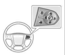
△ or ▽: Press to move up or down in a list. In the main view, you can press up and down to move between different info app pages.
