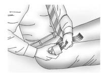
To make the belt longer, tilt the latch plate and pull it along the belt.
