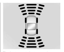
The instrument cluster may have a parking assist display with bars that show "distance to object" and object location information for RPA, and on some vehicles, for FPA. As the object gets closer, more bars light up and the bars change color from yellow to amber to red.
