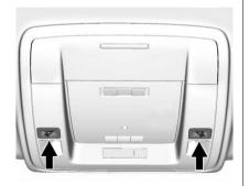
There are reading lamps in the overhead console and the headliner, if equipped. To operate, the ignition must be in the ACC/ACCESSORY or ON/RUN position or using Retained Accessory Power (RAP).
