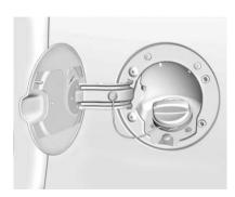
The fuel cap is behind a hinged fuel door on the driver side of the vehicle. Vehicles that have a FlexFuel badge and a yellow fuel cap can use either unleaded gasoline or ethanol fuel containing up to 85% ethanol (E85). See *E85* or FlexFuel on page 9-69.
