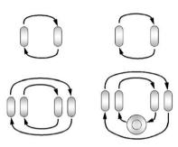
Use this rotation pattern when rotating the tires if the vehicle has polished forged aluminum dual rear wheels. The spare wheel can be used in any position and can be rotated with the rear inner wheels.
