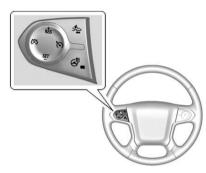
The Collision Alert control is on the steering wheel. Press to set the FCA timing to Far, Medium, Near, or Off. The first button press shows the current setting on the DIC. Additional button presses will change this setting. The chosen setting will remain until it is changed and will affect the timing of both the Collision Alert and the Tailgating Alert features. The timing of both alerts will vary based on vehicle speed. The faster the vehicle speed, the farther away the alert will occur.
