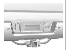
For vehicles equipped with heavy-duty trailering, the harness connector is mounted in the bumper. The seven-wire harness contains the following trailer circuits:
