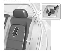
Pull the handle on top of the seatback to unlock it.
