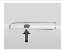
Touch the touch pad on a front door handle to lock the doors.
