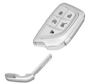
To remove the mechanical key, press the button near the bottom of the remote key, and pull the key out. Never pull the mechanical key out without pressing the button.
