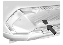
Carefully open the cover on the fascia by using the small notch that conceals the tow eye socket.
