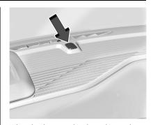
When the charge cord is plugged in, a color appears to indicate the charging status.
