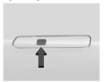
When the doors are unlocked and the remote key is within 1 m (3 ft) of a front door handle, touch the lock pad on a front door handle to lock the doors.
