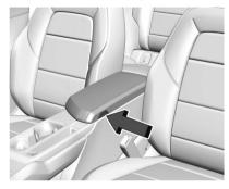
There is storage in the center console. Lift the lever on the side to open.
