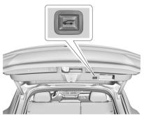
When closing the liftgate, press the button on the bottom of the gate.
