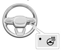
: Press to turn the heated steering wheel on or off. An indicator next to the button is lit when the feature is turned on.
