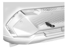
Install the tow eye into the socket and turn it until it is fully tightened. When the tow eye is removed, reinstall the cover with the notch in the original position.
