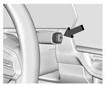
This position locks the drive wheels. Use P (Park) when starting the vehicle to ensure the vehicle does not move.
