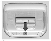
: Press this button on the overhead console to make the front and rear turn signal lamps flash on and off. This warns others that you are having trouble. Press again to turn the flashers off.
