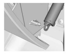
Disconnect the glove box door damper
