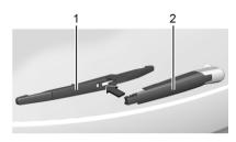
Align the new wiper blade assembly (1) with the wiper arm (2) and install by pushing up on the wiper blade assembly until it clicks into place on the wiper arm.
