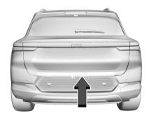
To open the liftgate, press the touch pad.
