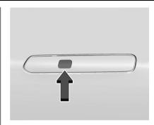
Touch the lock pad on a front door handle to lock the doors.
