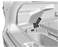
Insert the SD card into the card reader in the rear compartment. Disable the system from the playback screen before removing the SD card from the reader. Do not remove the card while recording is enabled. This could corrupt the video file and/or the SD card.
