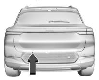
To access the liftgate key lock cylinder, remove the cover plug and insert the mechanical key into the cylinder. Turn to unlock. See *Keys* ⋄ 8.
