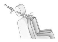
If the position you are using has an adjustable headrest or head restraint adjust it accordingly to allow proper fitment. If you are using a dual tether, route the tether in between the headrest or head restraint posts.
