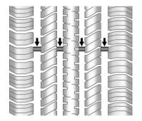
Treadwear indicators are one way to tell when it is time for new tires. Treadwear indicators appear when the tires have only 1.6 mm (1/16 in) or less of tread remaining. See *Tire Inspection* ⇒ 298 and *Tire Rotation* ⇒ 299.
