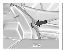
Stow the seat belt latch plate in the stowage slot.
