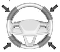
If your vehicle is equipped with Super Cruise, hold the steering wheel in the areas shown to help prevent undesired take steering alerts.
