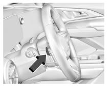
Regen on Demand allows for increased deceleration by pressing and holding the steering wheel paddle. Regen on Demand works in D (Drive). The accelerator pedal can be used to manage deceleration while using Regen on Demand. See One-Pedal Driving № 174.
