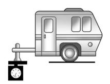
The trailer tongue weight contributes to the Gross Vehicle Weight (GVW). GVW includes the CURB WEIGHT of your vehicle, any passengers, cargo, equipment and the trailer tongue weight. Vehicle options, passengers, cargo, and equipment reduce the maximum allowable tongue weight the vehicle can carry, which also reduces the maximum allowable trailer weight.
