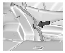
Ensure the seat belt latch plate is in the stowage slot.
