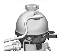
If the coolant level is not visible or needs to be adjusted within the reservoir, contact your dealer.
