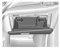
3. Squeeze both sides of the glove box bin inward to lower beyond the stops.
