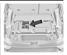
Thetire sealant can ister and compressor are secured with straps. Release the straps and remove the can ister and compressor.
