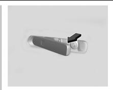
If the door is locked, touch the back of a front door handle to passively unlock the vehicle or press on the remote key. Pull the handle to open the door.
