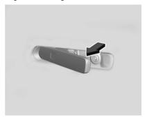
When the front door handles are pivoted outward, touch the back of a handle to unlock all doors.
