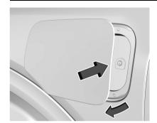
Push the rearward edge of the charge port door and release to open the door.
