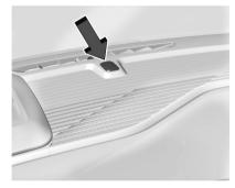
The light sensor is on top of the instrument panel. Do not cover the sensor.
