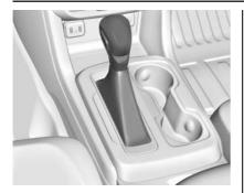
P: This position locks the drive wheels. Use P (Park) when starting the engine because the vehicle cannot move easily. When parked on a hill, especially when the vehicle has a heavy load, you might notice an increase in the effort to shift out of P (Park). See "Torque Lock" under Shifting Into Park ⇒ 188.
