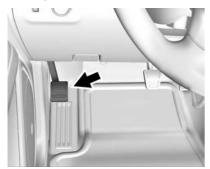
Set the parking brake by holding the regular brake pedal down, then pushing down the parking brake pedal.
