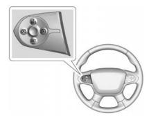
S: Press to turn the system on or off. A white indicator comes on in the instrument cluster when cruise control is turned on.
