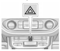
: Press to make the front and rear turn signal lamps flash on and off. Press again to turn the flashers off.
