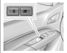
Press to activate the safety locks on the rear doors. The indicator light comes on when activated. The vehicle must be on, in ACC/ACCESSORY, or in Retained Accessory Power (RAP). See Retained Accessory Power (RAP) ⇒ 188.
