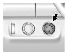
Use the transfer case shift knob, next to the steering wheel, to shift into and out of four-wheel drive for extra traction.
