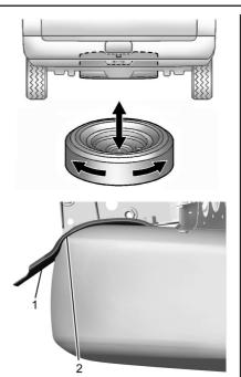
7. Make sure the tire is stored securely and flush in the radius (2) of the spare tire support bracket (1). Push, pull, and then
