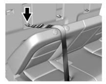
3.4. Adjust the top tether to its full length and attach the top tether hook to the anchor. Make sure that
