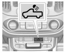
The exterior cargo lamps provide more light in the cargo area of the vehicle, if needed. The lamps inside the pickup box, tailgate handle, hitch, and the cargo mirror lamps also turn on, if equipped.
