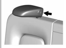
The rear outboard head restraints are designed to be folded. When folding the seatback down, the head restraint must first be manually folded forward out of the way to fold the seatback down.
