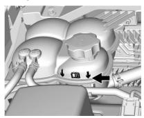
Check to see if coolant is visible in the coolant surge tank. If the coolant inside the coolant surge tank is boiling, do not do anything else until it cools down.
