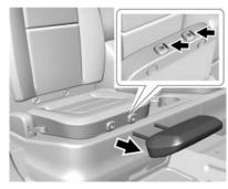
If installed as a seat cushion extension, first press both buttons on the front of the seat cushion to remove the headrest.
