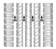
Treadwear indicators are one way to tell when it is time for new tires. Treadwear indicators appear when the tires have only 1.6 mm (1/16 in) or less of tread remaining. See *Tire Inspection* ⇔ 280 and *Tire Rotation* ⇔ 280 for additional information.
