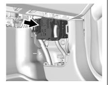
The instrument panel fuse block is behind the passenger side cowl side trim panel. Remove the plastic nut at the front of the cover, then pull the cover away from the trim panel to access the fuse block.
