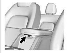
There is storage under the armrest in the center console. Press the button and lift.
