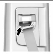
Push up on the release button and move the height adjuster to the desired position.
