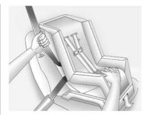
9. To tighten the belt, push down on the child restraint, pull the shoulder portion of the belt to tighten the lap portion of the belt, and feed the shoulder belt back into the retractor. When installing a forward-facing child restraint, it may be helpful to use your knee to push down on the child restraint as you tighten the belt.
