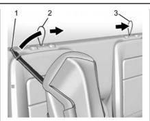
Route the top tether (1) through the loop (2) at the top of the seatback directly behind the child restraint and attach the top tether hook to the top tether loop at the top of the seatback for the opposite rear seating position (3).
