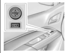
If equipped, adjust the power mirrors:
