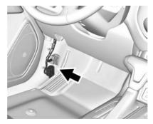
A four-wire harness, without connector, is secured behind the left side kick panel. The harness contains the following circuits:
