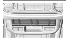
Turn the Tow/Haul Mode on and off by pressing the button on the center stack. When the Tow/Haul Mode is enabled, a light on the instrument cluster will come on.
