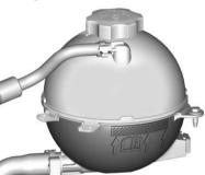
Check to see if coolant is visible in the coolant surge tank. If the coolant inside the coolant surge tank is boiling, do not do anything else until it cools down. See Engine Overheating
