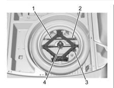
3. Turn the wing nut (4) counterclockwise to remove the jack (1), wheel wrench (2), and strap (3). Place the tool container near the tire being changed.
