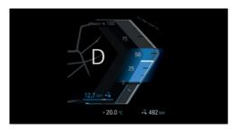
A blue range appears on the power gauge, indicating reduced electrical consumption while driving. Additionally, the bonus range will be displayed. The size of this blue range depends on the driving situation.
