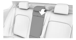
Pull lever and fold the center section forward.
