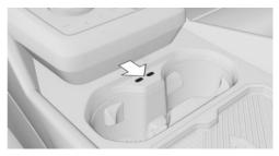
Two USB ports are located in the center console.
