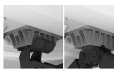
3. Extend the jack by turning the jack crank handle or lever clockwise.
