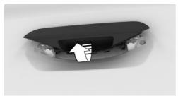
The position of the integrated key in the door lock depends on the vehicle.
