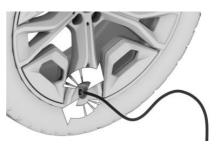
6. With the compressor switched off, insert the connector into the power socket in the vehicle interior.
