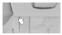
On the left side of the vehicle, there is a diagnostic socket for reading out vehicle data.
