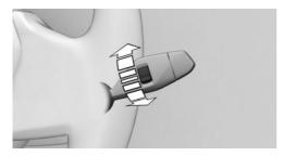
Turn the thumbwheel on the wiper lever.
