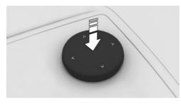
Slide the Controller in four directions to switch between menus, for example.
