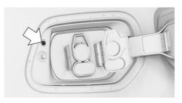
The charging cable release button is located next to the high-voltage charging socket.
