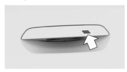
Touch the grooved surface on the door handle of a closed front door with your finger and hold it there without grasping the recessed grip.
