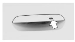
Touch the grooved surface on the external door handle of a closed front door with your finger and hold it there without grasping the recessed grip.
