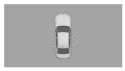
The maximum opening angle of the doors is displayed in selector lever position P.
