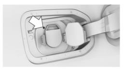
The charging status is shown by the indicator light on the high-voltage charging socket.
