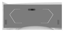
Depending on the equipment, the instrument cluster has up to three infrared light sources. Depending on the light conditions, these light sources can be visible when the vehicle is in standby mode.
