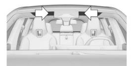
With climate comfort windshield: the marked area is not covered with heat-reflective coating.
