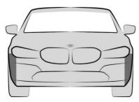
The radar sensors are located to the side in the front bumper.
