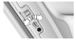
Unlock or lock the safety switch on the rear doors using the integrated key. To lock, turn in the corresponding arrow direction on the door.
