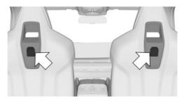
The mounts and USB ports are located behind the marked covers.
