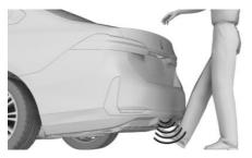
Moving a foot again will stop the opening proccedure. The subsequent foot movement will close the cargo area again.
