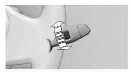
Turn the thumbwheel on the wiper lever.
