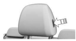
Press the button and push the head restraint up or down.
