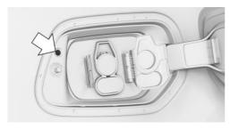
The charging cable release key is located next to the charging socket.
