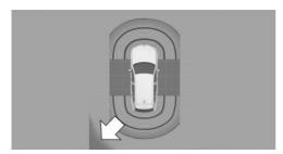
In the Park Distance Control view, the respective boundary area flashes red if vehicles are detected by the sensors.
