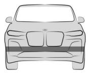
The ultrasonic sensors of the parking assistance systems are located in the front bumper.
