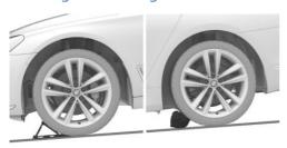
Place wheel chocks or other suitable objects, e.g., rocks, under the wheels of the front axle and rear axle, opposite the rolling direction.
