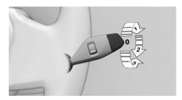
Turn the outer switch upward.
