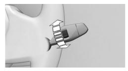
Turn the thumbwheel on the wiper lever.
