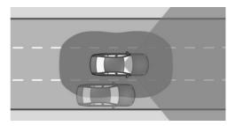
Radar sensors monitor the space next to the vehicle when traveling faster than a minimum speed and up to approx. 130 mph/210 km/h.
