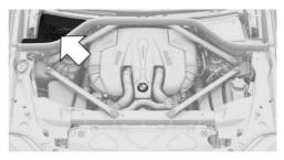
The battery for the Mild-Hybrid technology is located under a cover in the engine compartment on the front passenger side.
