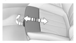
Pull the lever at the front of the seat and push the thigh support forward or back.
