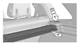
Press the release button, arrow 1, and pull the cargo cover out toward the rear, arrow 2.
