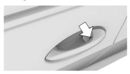
With your finger, touch and hold the grooved surface on a closed door handle without grasping the door handle.
