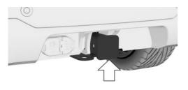
The mount for the trailer hitch is located on the rear of the vehicle.
