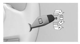
Turn the outer switch upward.
