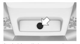
A socket is located in the center console. Detach the cover.
