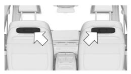
The mounts for attaching optional accessories are located behind the marked covers, as are the USB ports.
