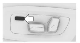
Press the button to reset to base position. The process is canceled if the button is pressed again.
