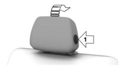
Press button, arrow 1, and fold the head restraint back.
