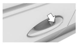
With your finger, touch and hold the grooved surface on a closed door handle without grasping the door handle.
