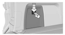
2. If necessary, remove the cargo cover from the storage under the cargo floor panel.
