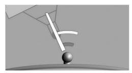
Two static circular segments help to estimate the distance of the trailer to the trailer hitch.
