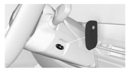
It is not possible to switch on the drive-ready state if the vehicle key has not been detected. Proceed as follows in this case:
