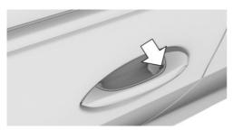
Touch the grooved surface on the external door handle of a closed front door with your finger and hold it there without grasping the door handle.
