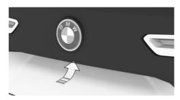
Press the button on the trunk to access the vehicle in deep sleep mode.
