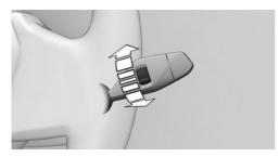
Turn the thumbwheel on the wiper lever.
