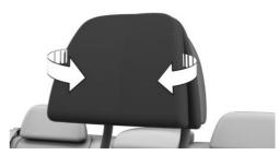
Fold the side extensions on the head restraint forward for increased side support in the resting position.
