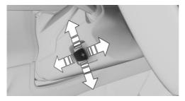
Press the switch to adjust the steering wheel forward/back position and height to the seat position.
