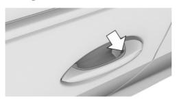
Touch the grooved surface on the external door handle of a closed front door with your finger and hold it there without grasping the door handle
