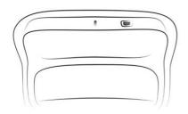
Press the button on the inside of the cargo area.
