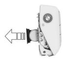
3. Remove the battery from the battery housing.
