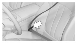
To ease accessibility to the safety belt buckle, an adjustable slider is available on the belt to help position the buckle when not in use.
