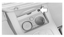
If the vehicle is equipped with thermo-cup holders, a USB port is located in the center console.
