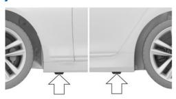
The jacking points for the vehicle jack are located at the indicated positions.
