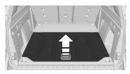
The onboard vehicle tool kit is located under the cargo floor panel.
