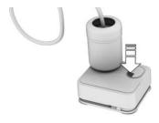
Let the compressor run for max. 10 minutes to fill the tire with sealing compound and achieve a tire inflation pressure of approx. 2.0 bar.
