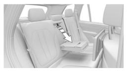
Fold down the center armrest and pull on the loop.
