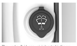
The washer fluid reservoir is located in the enaine compartment.
