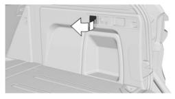
A socket is located on the right side in the cargo area. Unfold the cover.
