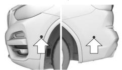
The ultrasound sensors of the Automatic Parking Assistant are located on the side of the vehicle.
