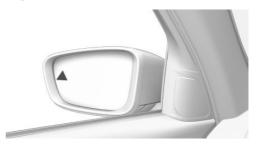
The light in the exterior mirror flashes if vehicles are detected by the rear sensors and your own vehicle is moving in reverse.
