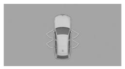
The maximum opening angle of the doors is displayed in selector lever position P. As soon as the vehicle begins moving, the opening angles are replaced by parking aid lines.
