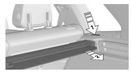
Press the release button, arrow 1, and pull the cargo cover out toward the rear, arrow 2.
