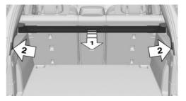
Pull out the cargo cover, arrow 1, and hook both sides into the brackets, arrow 2.
