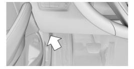
Located on the driver's side is an OBD socket for reading the vehicle data.
