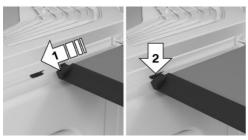
To restore the functionality, close the cargo cover by hand, arrow 1, until it engages in the mounting, arrow 2.
