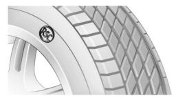
The tires are marked on the tire sidewall with Run-flat System Component RSC.
