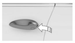
2. Guide one finger of your other hand from the back under the cover and push the cover out. Use the thumb for counter support to prevent the cover from falling out of the door handle.
