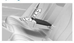
Press the button, arrow 1, and fold the cover up, arrow 2.
