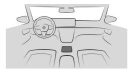
The Controller is located in the center console.
