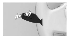
➤ To turn on the high-beam headlights, push the turn signal lever forward, arrow 1. The high-beam headlights illuminate when the low-beam headlights are switched on.
