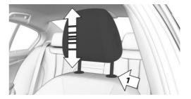
To lower the height of the head restraint, press the release button on the backrest, arrow 1, then push the head restraint down-
