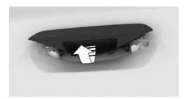
2. Unlock the door lock with the integrated key by turning it counterclockwise.
