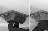
3. Extend the jack by turning the jack crank handle or lever clockwise.
