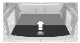
To open the storage compartment, use the handle to pull the cargo area floor upward and fold it forward.
