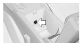
A socket is provided in the front center armrest under a cover. Pull off the cover before using the socket.
