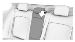
Pull down the sliding button to the right of the head restraint and fold the center section forward.
