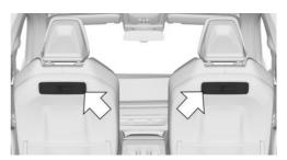
The mounts are located on the front seat backrests, behind the marked covers.
