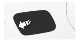
2. Open the fuel filler cap counterclockwise.
