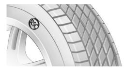
Runflat tires are labeled with a circular icon containing the letters RSC marked on the tire sidewall.
