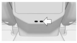
Two USB ports are located in the rear center console.
