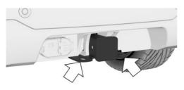
Two eyes can be found on the mount for the trailer hitch for attaching the trailer safety chain.
