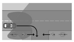
In addition, the sensors detect the traffic situation in their detection range when turning.
