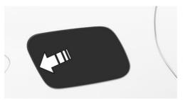
2. Turn the fuel filler cap counterclockwise.
