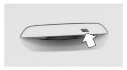
Touch the grooved surface on the external door handle of a closed front door with your finger and hold it there without grasping the recessed grip.
