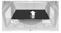
Fold out the cargo area floor holder in order to hold the cargo area floor in the folded-up position.
