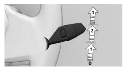
To activate the rain sensor: Push the wiper lever upward from position 0, arrow 1, once. Wiping operation is started.
