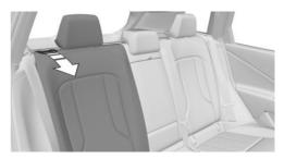
Pull the lever in the recess and fold the rear seat backrest forward.
