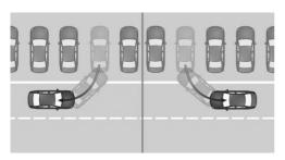
When driving out of perpendicular parking spaces.
