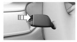
Continue to press the button on the turn signal lever until the desired widget is selected.
