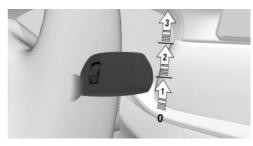
Activate: press the lever up once from its 0 position, arrow 1.
