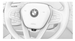
Button for steering wheel heating
