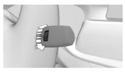
Turn the thumbwheel to adjust the sensitivity of the rain sensor.
