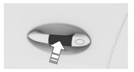
Hold the near field communication antenna of the smartphone directly and centered on the external door handle of the driver's door.
