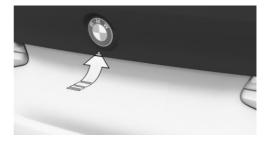
Press the button on the outer side of the tailaate.
