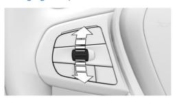
Press the rocker switch up or down repeatedly until the desired speed limit is set.
