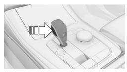
3. Push the selector lever in the desired direction, past a resistance point, if needed. The selector lever automatically returns to the center position when released.
