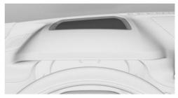
The protective glass of the Head-up display is located in the position marked.
