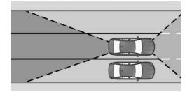
Radar sensors monitor the space next to the vehicle when traveling faster than a minimum speed and up to approx. 130 mph/210 km/h.
