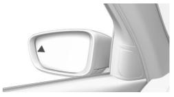
The warning light in the exterior mirror warns of a possible collision with a detected vehicle.
