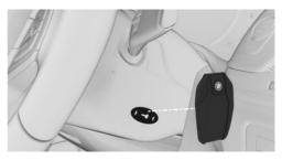
It is not possible to switch on the drive-ready state if the display key has not been detected.
