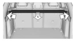
Pull out the cargo cover, arrow 1, and hook both sides into the brackets, arrow 2.
