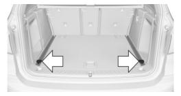
To secure the cargo there are additional movable lashing eyes in the cargo area.
