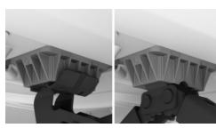
3. Extend the jack by turning the jack crank handle or lever clockwise.
