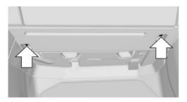
Loosen fasteners, arrows, and open cover.
