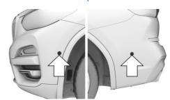
The ultrasonic sensors for Parking Assistant are located to the side in the front and rear bumpers.
