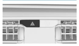
The button is located in the center console. The red light in the button flashes when the hazard warning flashers are activated.
