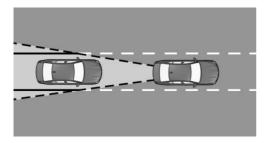
Radar sensors monitor the area behind the vehicle.
