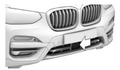
The front radar sensor is located in the front bumper.
