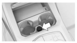
A socket is located between the cup holders. Detach the cover.
