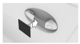
Hold activated Key Card directly on the center of the external door handle of the driver's door. If the Key Card is not detected, slightly change the position of the Key Card and repeat the
