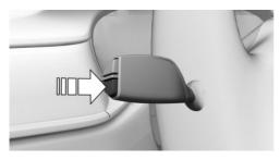
Press the button on the turn signal lever.
