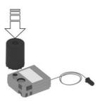
2. Turn the sealant bottle clockwise by 90° to the stop.
