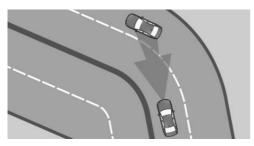
When you approach a curve the system may briefly report vehicles in the next lane due to the bend of the curve. If the system decelerates you may compensate for it by briefly accelerating. After releasing the accelerator pedal the system is reactivated and controls speed independently.
