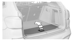
Lift the cargo area floor up until it is over the multifunction hook.
