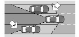
Radar sensors monitor the area behind and next to the vehicle when traveling faster than a minimum speed.
