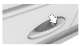
Touch the grooved surface on the handle of a closed vehicle door with your finger for approx. 1 second without grasping the door handle.
