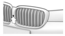
The front camera is located in the radiator arille.
