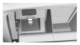
3. Remove the cover of the fragrance cartridge. Hold the cover on the top to slide it from the fragrance cartridge.
