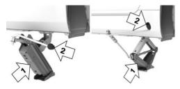
2. Insert the jack into the rectangular recess of the jacking point closest to the wheel to be changed.
