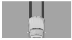
The car wash view assists when entering a car wash by displaying the floor and the vehicle's own track.
