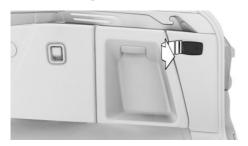
Pull the corresponding lever in the cargo area to release the rear seat backrest.
