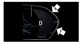
Needle in the area of arrow 1: display of the energy recovered by coasting or when decelerating, CHARGE.
