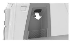
Open the bracket and take the warning triangle out in the direction of the car's interior.
