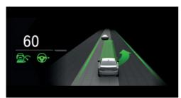
An example: the indicator and warning lights for the Active Cruise Control with Stop&Go function and the Lane Change Assistant indicate a lane change to the next lane. At the same time, the lane change to the next lane is shown with animation in the Assisted Driving View.
