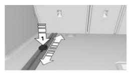
To shift the lashing eyes, press the button, arrow 1. Make sure that the lashing eyes latch at the new position.
