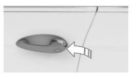
2. Guide one finger of your other hand from the back under the cover cap and push the cover cap out.
