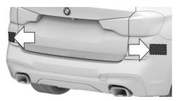
The radar sensors are located to the side behind the rear bumper.
