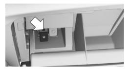
6. Slide the fragrance cartridge into the cartridge holder at a slight angle without applying pressure. The fragrance cartridge is correctly positioned when the cartridge holder can be closed.
