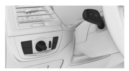
The light switch is located next to the steering wheel.
