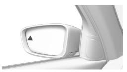
The warning light in the exterior mirror flashes if the rear sensors detect other vehicles when the vehicle is reversing.
