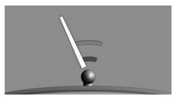
Two static circle segments show the distance between the trailer and the trailer hitch
