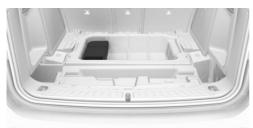
The Mobility System is located in the compartment under the cargo floor panel.
