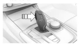
Push the selector lever in the desired direction, past a resistance point, if needed. The selector lever automatically returns to the center position when released.
