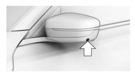
One camera is located at the bottom of each exterior mirror housing.
