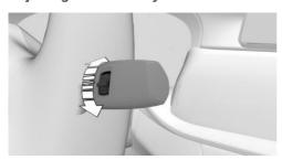
Turn the thumbwheel on the wiper lever.
