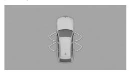
Steptronic transmission: the maximum opening angles of the doors are displayed in selector lever position P.
