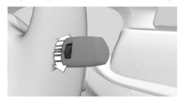
Turn the thumbwheel to adjust the sensitivity of the rain sensor.
