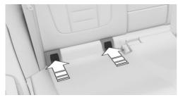
Attach to the lower LATCH anchors located behind the indicated covers.
