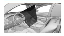
The gestures that are performed underneath the interior mirror are captured by a camera in the roofliner
