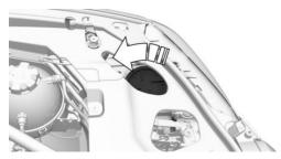
3. Pull the bulb holder out past the spring resistance point.
