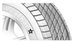
For each tire size, the manufacturer of the vehicle recommends certain tire brands. The tire brands can be identified by a star on the tire sidewall.
