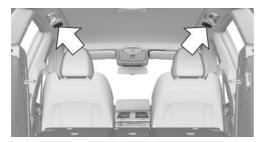
Insert each of the two top retaining pins of the cargo area partition net into the receptacles until they reach the stop, arrow 1, and push them forward.
