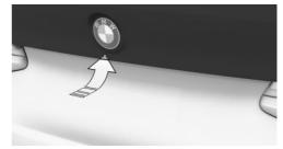
▶ Unlock the vehicle and then press the button on the outside of the tailgate.
