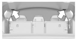
Insert each of the two top retaining pins of the cargo area partition net into the receptacles until they reach the stop, arrow 1, and push them forward.
