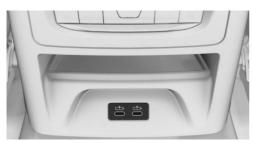
A USB interface with two USB ports is located in the center console in the rear.
