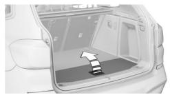
2. Lift the cargo floor panel up until it is over the multi-function hook.
