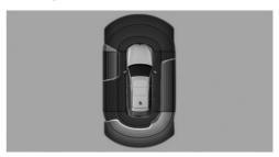
To protect the sides of the vehicle, obstacle markings are displayed on the sides of the vehi-
