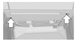
Loosen fasteners, arrows, and open cover.
