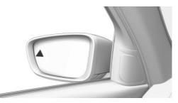
The light in the exterior mirror flashes if vehicles are detected by the rear sensors and your own vehicle is moving backwards.
