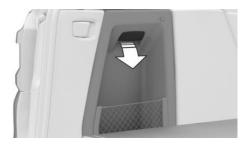
Open the bracket and take the warning triangle out in the direction of the car's interior.
