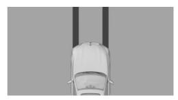
The vehicle wash view assists when entering a vehicle wash by displaying the floor and the vehicle's own track.
