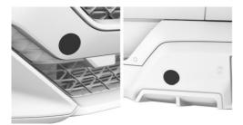
The towing eye thread is located behind a cover on the front and rear bumper.
