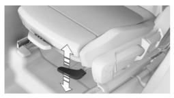
To adjust the seat tilt: On the front of the seat, push the seat tilt lever up or down as many times as necessary for the seat to reach the desired tilt.
