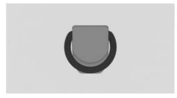
The lashing eyes are located on the side panels in the cargo area.
