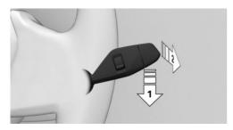
To turn off the wiper system, push the wiper lever down until it reaches position 0, arrow 1.
