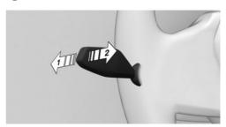
➤ To turn on the high-beam headlights, push the turn signal lever forward, arrow 1. \*
