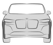
The radar sensors are located on the side of the front bumper.
