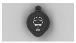
The washer fluid reservoir is located in the engine compartment on the right side of vehicle.
