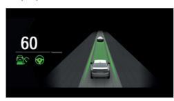
An example of active Driver Assistance: the indicator and warning lights for Distance Control and Assisted Driving Mode are displayed. At the same time, the Distance Control is animoted in Assisted View.
