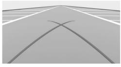
The turning circle lines show the path with the smallest possible turning circle on level roads in the camera image on the control display.
