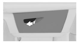
To open the glove compartment, pull the glove compartment handle.
