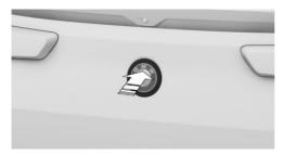
Press the top half of the BMW emblem on the cargo area to access the vehicle while in deep sleep mode. Deep sleep mode remains on in this case.
