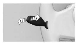
To reactivate the High Beam Assistant, press the turn signal lever up, arrow 1.
