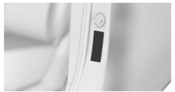
The tire inflation pressure specifications can also be found on the tire pressure label on the driver's door pillar.
