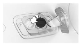
3. Place the fuel filler cap in the mount on the fuel filler flap.
