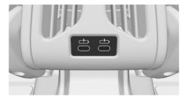
Depending on vehicle equipment, the back of the center console will have one or two USB ports.
