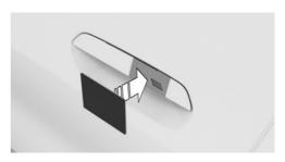
Hold the activated Service Card directly over the middle of the driver's door handle.
