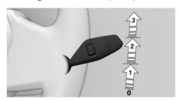
To turn on the wiper system, push the wiper lever upward to the desired position.
