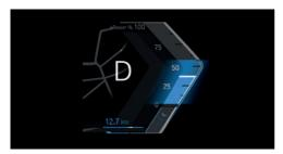
The efficient range of the power gauge is colored blue. Additionally, the bonus range will be displayed.
