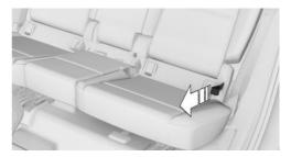
Pull the loop on the side of the seat and fold the rear seat backrest forward.
