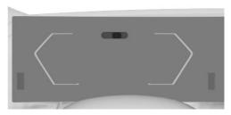
Depending on vehicle equipment, the instrument cluster may have some infrared light sources. Depending on the light conditions, these light sources can be visible when the vehicle is in standby mode.
