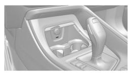
The USB port is located in the front center console.
