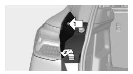
3. Loosen both nuts, arrow 1, of the outer tail light. Use the handle of the screwdriver from the onboard vehicle tool kit to loosen.
