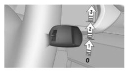
To activate: press the lever up once from its basic setting, arrow 1.
