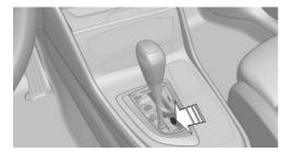
Press the button on the front of the selector lever and move the selector lever back slightly.
