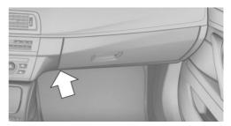
The socket is located below the glove compartment.
