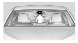
The comera is installed near the interior mirror.
