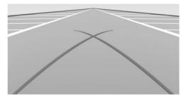
Turning circle lines can only be superimposed on the rearview camera image together with pathway lines.
