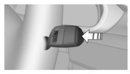
Press the button on the wiper lever.
