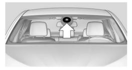
The camera is installed near the interior mirror. Keep the windshield in front of the interior mirror clean and clear.
