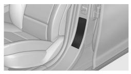
These tire inflation pressure values can also be found on the tire pressure label on the driver's door pillar.
