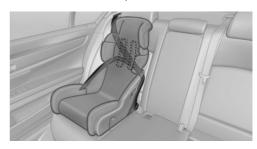
The rear seat belts and the front passenger seat belt can be permanently locked to fasten child restraint systems.
