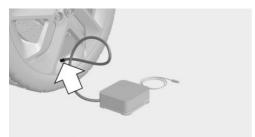
3. Insert the connector into the power socket in the vehicle interior.
