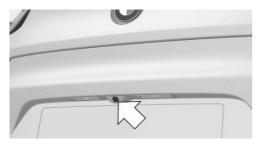
The camera lens is located between the license plate lights.
