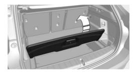
Grasp the cargo floor panel in the rear and fold up above the locking point of the upper position, refer to page 207. 3. Pull the cargo floor panel backward from the brackets.
