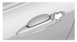
Touch the surface on the door handle of the driver's or front passenger door, arrow, with your finger and hold it there without grasping the door handle.
