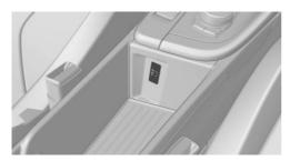
The USB port is located in the center console.
