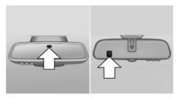
Photocells are used for control:
