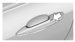
Touch the surface on the door handle of the driver's or front passenger door with your finger for approx. 1 second without grasping the door handle.
