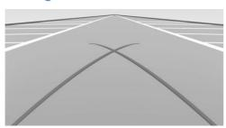
Turning radius lines can only be superimposed on the rearview camera image together with pathway lines.
