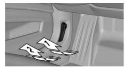
2. After the lever is released, pull the lever again, arrow 2.
