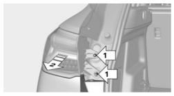
4. Pull the plug out of the bulb holder and have the tail light wiring hang outside.
