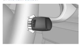
Turn the thumbwheel to adjust the frequency or sensitivity of the rain sensor.
