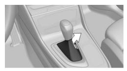
Lift the sleeve. Unplug the cable connector, if needed.  Using the screwdriver from the onboard vehicle tool kit, refer to page 262, press the yellow release lever downward, arrow.
