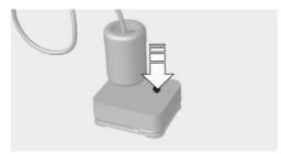
Let the compressor run for max. 10 minutes to fill the tire with sealant and achieve a tire inflation pressure of approx. 2.0 bar.
