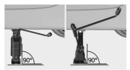
Crank the vehicle up, until the vehicle jack is with the entire surface on the ground and the relevant wheel is maximum 1.2 inches/3 cm above ground.
