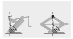
Make sure that the vehicle jack foot stands vertically and perpendicularly beneath the jacking point after extending the vehicle jack.
