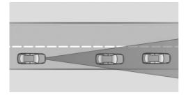
The detection capacity of the system and the automatic braking capacity are limited.
