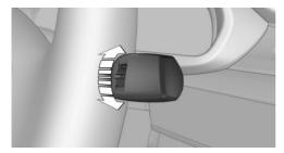
Turn the thumbwheel on the wiper lever.
