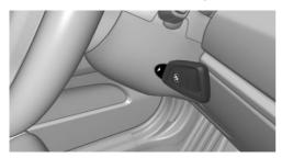
It is not possible to start the engine if the vehicle key has not been detected.
