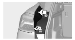
Loosen both nuts, arrow 1, of the outer tail light. Use the handle of the screwdriver from the onboard vehicle tool kit to loosen.
