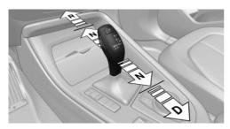
The selector lever positions R, N, and D are selected by tapping the selector lever forward or
