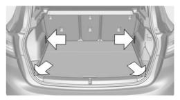
With cargo area partition net or ski and snowboard bag: to secure the cargo there are six lashing eyes in the cargo area.
