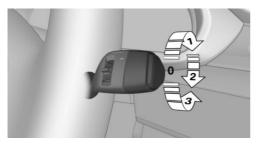
Turn the outer switch upward.
