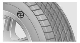
The tires are marked on the tire sidewall with RSC Run-flat System Component.
