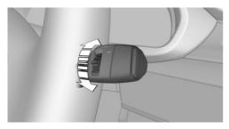
Turn the thumbwheel on the wiper lever.
