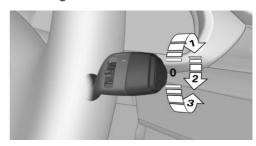
Turn the outer switch upward.
