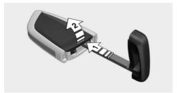
Push battery in the direction of the arrow using a pointed object and lift it out.
