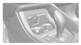
The USB port is located in the front center console.
