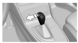
Press the selector lever to the left out of selector lever position D.
