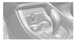
The USB interface is located in the front center console.
