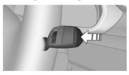
Press the button on the wiper lever.
