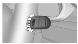
Turn the thumbwheel on the wiper lever.
