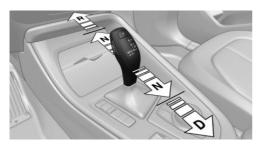
The selector lever positions P, R, N, and D are selected by tapping the selector lever forward or
