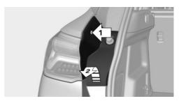
3. Loosen both nuts, arrow 1, of the outer tail light. Use the handle of the screwdriver from the onboard vehicle tool kit to loosen.
