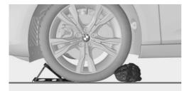
Place chocks or other suitable objects, for example a rock, in front of and behind the wheel that is diagonally opposite to the wheel that you wish to change.
