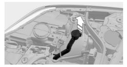
Turn the bulb socket counterclockwise and remove.
