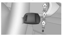
To activate: press the lever up once from its standard position, arrow 1.
