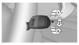
Turn the outer switch upward.
