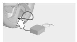
Insert the connector into the power socket inside the vehicle.
