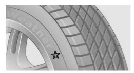
For each tire size, the manufacturer of the vehicle recommends certain tire brands. The tire brands can be identified by a star on the tire sidewall.
