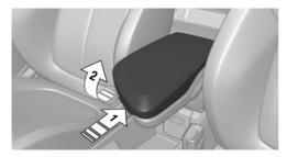
Pull the lever, arrow 1, and fold the center armrest up, arrow 2.
