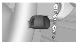
Press the lever up once from its standard position, arrow 1.
