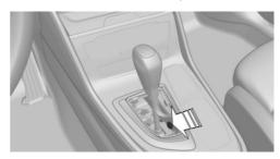
Press the button on the front of the selector lever and move the selector lever back slightly.
