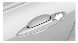
Touch the surface on the door handle of the driver's or front passenger door with your finger for approx. 1 second without grasping the door handle.
