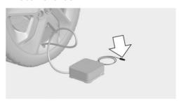
5. With the ignition switched on or the engine running, switch on the compressor.
