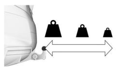
The permissible gross weight of the loaded rear carrier depends on how far its center of gravity is from the ball head.
