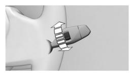
To adjust the sensitivity of the rain sensor, turn the knurled wheel on the wiper lever.
