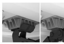
3. Extend the jack by turning the jack crank handle or lever clockwise.
