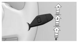
To turn on the wiper system, push the wiper lever upward to the desired position.
