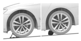
If it is necessary to change a wheel on a slight downhill gradient, place chocks and other suitable objects, e.g., rocks, under the wheels of the front and rear axles, against the direction that the vehicle will move.
