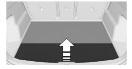
To open the storage compartment, grip the rear edge of the cargo area floor and fold it forward.
