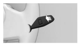
To clean the windshield, pull the wiper lever back.
