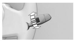
To adjust the sensitivity of the rain sensor, turn the knurled wheel on the wiper lever as follows:
