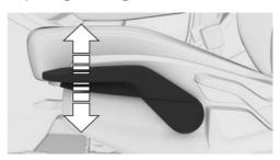
To adjust the height: On the side of the seat, push the front seat height lever up or down as many times as necessary for the seat to reach the desired height.
