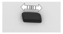
To adjust the longitudinal direction, push the longitudinal direction switch on the seat forward or backward.
