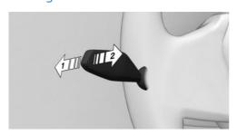
To turn on the high-beam headlights, push the turn signal lever forward, arrow 1. The high-beam headlights illuminate when the lowbeam headlights are switched on.
