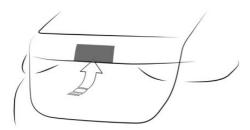
▶ Unlock the vehicle, then press the Open button on the outside of the cargo area.
