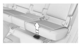
To adjust the longitudinal direction of the second row seats, pull the longitudinal direction lever at the front of the seat and push the seat in the desired direction.
