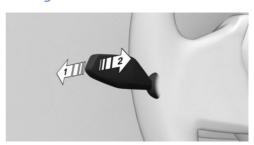
➤ To turn on the high-beam headlights, push the turn signal lever forward, arrow 1. \*
