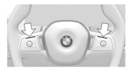
Similar to the displays for Assisted Driving Mode on the instrument cluster, the two LEDs above the keypads on the steering wheel illuminate.
