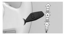
To activate the rain sensor: Push the wiper lever upward from position 0, arrow 1, once.
