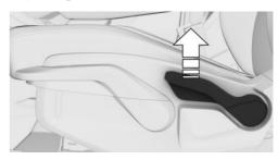
To adjust the backrest angle, pull the backrest tilt lever on the side of the seat and tighten or loosen the backrest as required.
