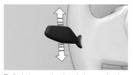
To flash the turn signal, push the turn signal lever up or down past the resistance point.
