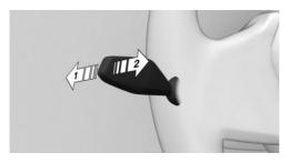
Press the turn signal lever forward, arrow 1, or pull the turn signal lever backward when the high-beam headlights are on, arrow 2.
