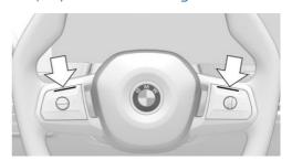
The two LEDs above the keypads on the steering wheel illuminate depending on the situation.
