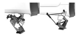
4. Take your hand away from the jack as soon as the lack is under load and continue turning the jack crank handle or lever with one hand.
