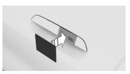
Hold the activated Key Card directly at the center of the driver's door handle.
