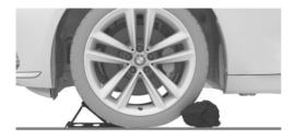
Place chocks or other suitable objects in front and behind the wheel that is diagonal to the wheel being changed.
