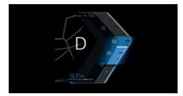
The efficient range of the power gauge is colored blue. Additionally, the bonus range will be displayed.
