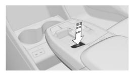
Press the parking brake button on the center console.
