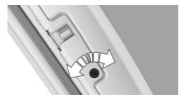
To secure the rear doors, release/lock the safety switch on the rear door using the integrated key.
