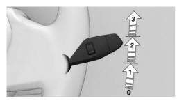
To activate the rain sensor: Push the wiper lever upward from position 0, arrow 1, once. To deactivate the rain sensor: Push the wiper
