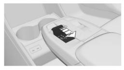
To activate LOW mode, pull the selector lever from selector lever position D to  $\mathrm{D}/\mathrm{L}$ .
