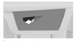
Pull the handle on the glove compartment.
