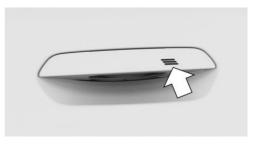
To close a window using the door handle of a closed front door, place a finger on the grooved surface of the door handle and hold it there without reaching into the recessed grip.
