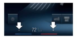
You can set the desired temperature for driver and front passenger individually on the menu
