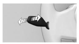
To reactivate the Automatic High Beam Assistant, press the turn signal lever up, arrow 1.
