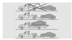
The vehicle should be transported with a tow truck with a so-called spectacle lift or on a loadina platform.
