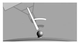
Two static circle segments are displayed in the camera image. These circle segments help to estimate the distance of the trailer to the trailer hitch
