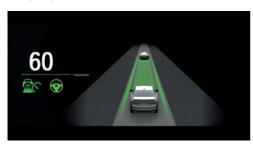
An example of active Driver Assistance: the indicator and warning lights for Distance Control and Assisted Driving Mode are displayed. At the same time, the Distance Control is animated in Assisted View.
