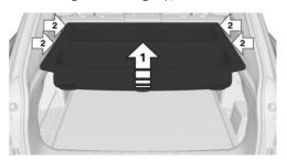
3. Firmly pull the cover backward out of the brackets, arrow 2.
