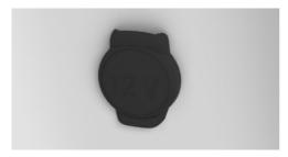
A socket is located on the right side in the cargo area. Unfold the cover.
