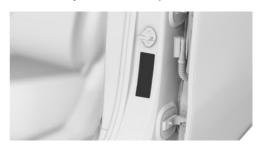
The tire inflation pressure specifications can also be found on the tire pressure label on the driver's door pillar.
