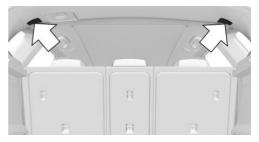
3. Insert each of the two top retaining pins of the cargo area partition net into the receptacles until they reach the stop, arrow 1, and push them forward.
