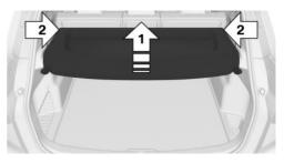
3. Firmly pull the cover backward out of the brackets, arrow 2.
