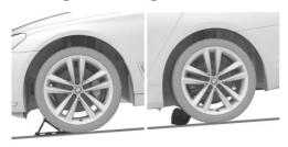
If you need to change a wheel on a slight downhill grade, place chocks and other suitable objects, for instance rocks, under the proper side of the wheels of both the front and rear axles to block the car from rolling downhill.
