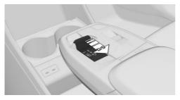
To activate the Sport program, pull the selector lever from selector lever position D to D/S.
