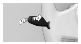
To turn on the high-beam headlights, push the indicator/high-beam stalk forward, arrow 1. The high beams illuminate when the low beams are switched on.
