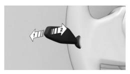
Press the indicator/high-beam stalk forward, arrow 1, or pull the high-beam stalk backward when the high beams are on, arrow 2.
