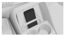
Insert your mobile phone upright and in the center, behind the retaining clip, and slide it down to the stop. The mobile phone display must point upwards.
