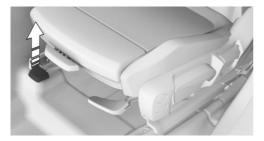
At the front of the seat, pull the lever for the longitudinal direction and push the seat in the desired direction.
