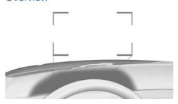
Head-up display views are projected onto the windshield through a protective glass. The protective glass is located between the steering wheel and windshield.
