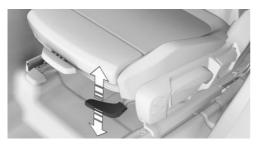
At the front of the seat, push the seat angle lever up or down as often as needed until the seat has reached the desired inclination.
