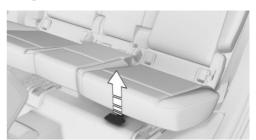
At the front of the seat, pull the lever for the longitudinal direction and push the seat in the desired direction.
