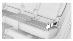
Pull the loop on the side of the seat and fold the rear seat backrest forward.
