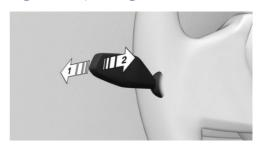
To turn on the high-beam headlights, push the indicator/high-beam stalk forward, arrow 1. \*
