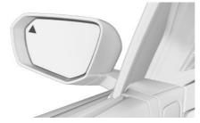
The warning light in the exterior mirror flashes if the rear sensors detect other vehicles when the vehicle is reversing.
