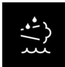
A yellow warning light is illuminated in the instrument cluster: fill level too low. The remaining range is displayed in the instrument cluster. Immediately add at least 1.3 US gal/5 liters of diesel exhaust fluid.
