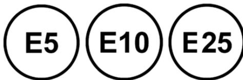
When using minimum quality fuel like RON 91 or fuel with an ethanol content of more than 10% to max. 25%, knocking noises may occur and driving and acoustic performance may change. These have no effect on the engine service life.
