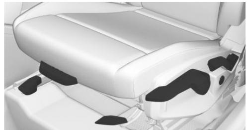
The levers for setting the seats are located on the front seats.
