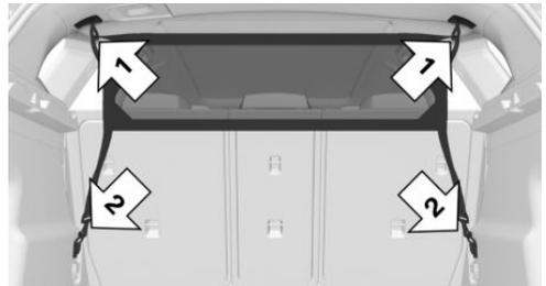
4. Use the two lower hooks to hook the cargo area partition net into the lashing eyes in the cargo area, arrow 2.
