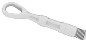
The screw-in tow fitting should always be carried in the vehicle.
