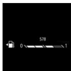
An arrow beside the fuel pump icon shows which side of the vehicle the fuel filler flap is on.
