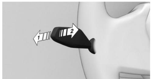
Press the turn signal lever forward, arrow 1, or pull the turn signal lever backward when the high beams are switched on, arrow 2.
