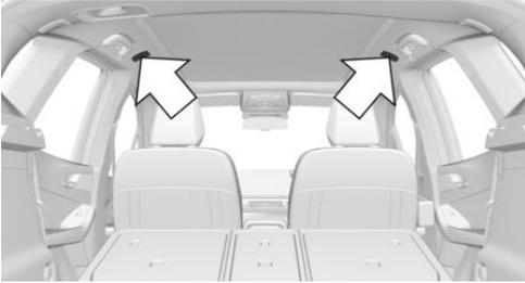
3. Insert each of the two top retaining pins of the cargo area partition net into the receptacles until they reach the stop, arrow 1, and push them forward. Make sure that the bottom hooks point to the front.
