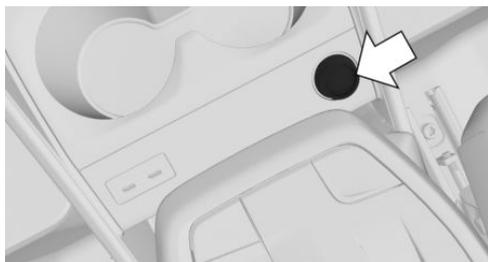
A socket is located between the smartphone tray and the cup holders. Detach the cover.
