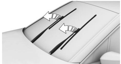
3. Press the button, arrow 1, turn the wiper blade slightly clockwise, and pull it forward and out, arrow 2.
