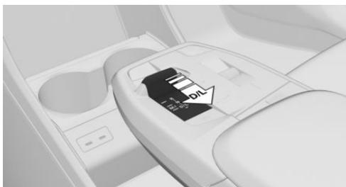
Pull the selector lever from selector lever position D to D/L.
