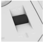
Press and hold the thumbwheel in the center console until the OFF indicator in the instrument cluster goes out.
