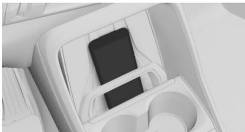
Insert the mobile phone upright and in the center behind the retaining clip and slide it down to the stop. The mobile phone display must point upwards.
