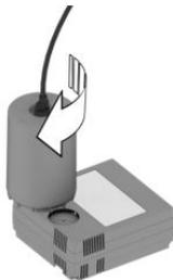
4. Unscrew the valve cap from the wheel and screw the connecting piece of the filler hose onto the valve.
