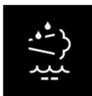
Tank for diesel exhaust fluid is empty. Immediately add at least 4 US gal/15 liters of diesel exhaust fluid. The engine will continue to run as long as it is not switched off and all other operating conditions are satisfied; sufficient fuel, for instance.
