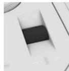
Press thumbwheel in the center console. The control display and the instrument cluster illuminate.
