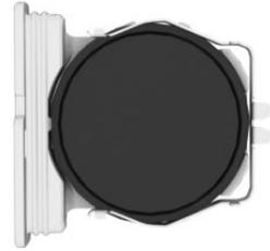
4. Insert a CR2032 3V battery with the positive side facing down.
