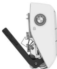
3. Remove the integrated key from the vehicle key.
