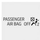
The indicator light is continuously illuminated when the seat is not occupied or when a child is detected on the seat in a provided child restraint system as intended. The airbags on the passenger's side are not activated.
