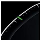
A mark is displayed on the speedometer for the set speed.
