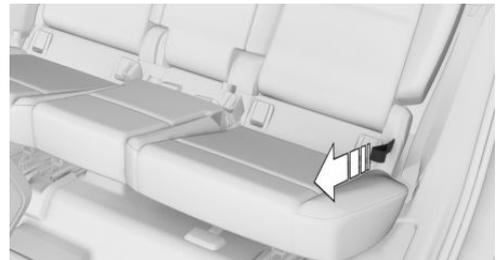
Pull the loop and fold the rear seat backrest forward.
