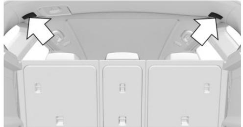
3. Insert each of the two top retaining pins of the cargo area partition net into the receptacles until they reach the stop, arrow 1, and push them forward.
