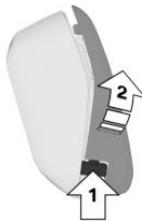
2. Remove the battery housing from the vehicle key to the side.
