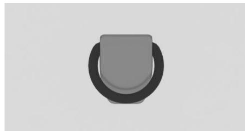
The lashing eyes are located on the loading sill and on the side walls of the trunk.
