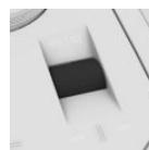
Press thumbwheel in the center console. The control display and the instrument cluster illuminate.
