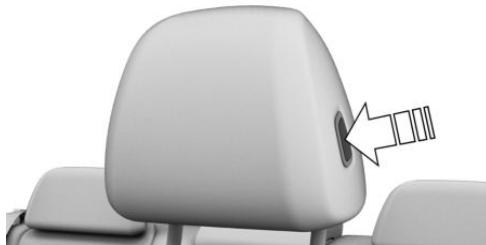
Press the button and push the head restraint forward or backward.
