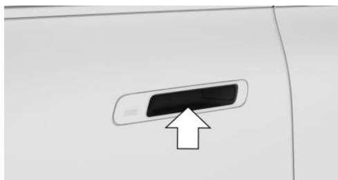
Reach into the recessed grip of the door and pull the door outward.
