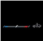
▷ Cold engine: the needle is in the blue temperature range, close to the stop of the temperature display, and the word WARM-UP is displayed.
