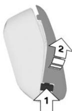
2. Slide out the integrated key at the open side of the vehicle key.
