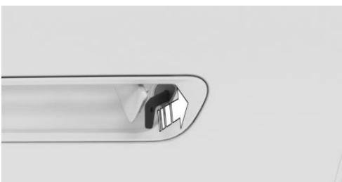
4. Remove the integrated key from the door lock.
