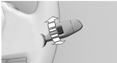
Turn the thumbwheel on the wiper lever.
