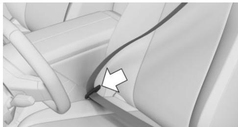
When the seat belt is fastened, the driver's and front passenger's belt straps are automatically tightened once after driving away.
