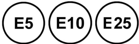
When using minimum quality fuel like RON 91 or fuel with an ethanol content of more than 10% to max. 25%, knocking noises may occur and driving and acoustic performance may change. These have no effect on the engine service life.
