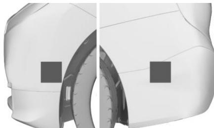
The ultrasonic sensors of the parking assistance systems are located on the side in the front and rear bumpers.
