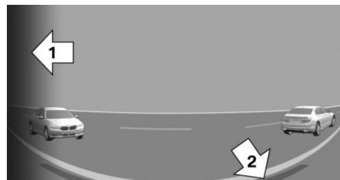
Depending on the direction of travel, the view to the front or back is displayed in the camera image.
