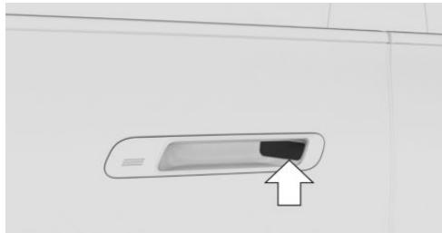
2. Pull the cover cap to the side so that the door lock is clearly visible.
