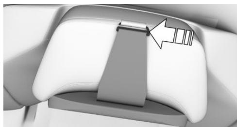
2. Bring the head restraint to a sufficiently high position.
