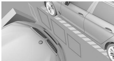
To protect the sides of the vehicle, obstacle markings are displayed on the sides of the vehicle.
