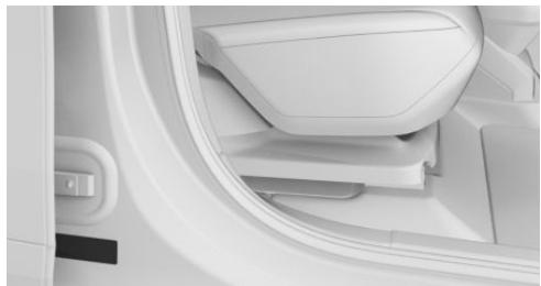
The vehicle identification number can be found on the nameplate, on the right-hand side of the vehicle.
