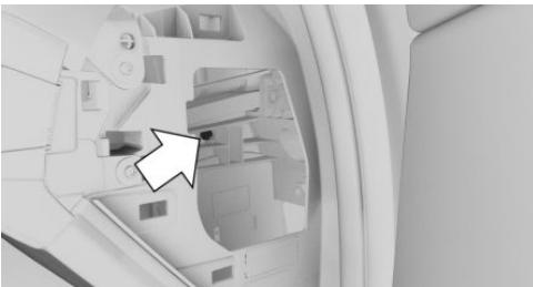
5. Pull the object out of the opening again. The glove compartment opens.
