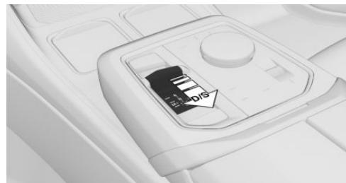
Pull the selector lever from selector lever position D to D/S.
