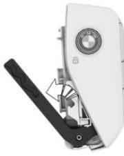
3. Remove the integrated key from the vehicle key.
