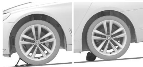
If you need to change a wheel on a slight downhill grade, place chocks and other suitable objects, for instance rocks, under the proper side of the wheels of both the front and rear axles to block the car from rolling downhill.
