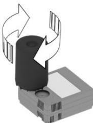
3. Connect the filler hose to the outlet of the sealant bottle and turn clockwise by 90° to the stop.
