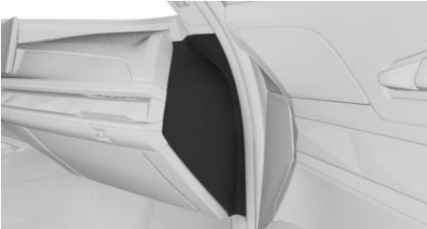
3. Press the sound insulation downward or remove it.
