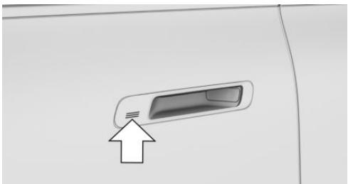
Touch the grooved surface on the external door handle of a closed front door with your
