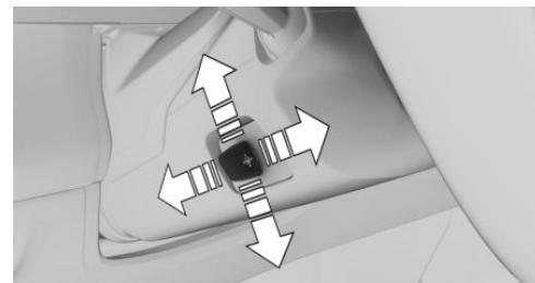
Press the switch to adjust the forward/back position and height of the steering wheel to the seat position.
