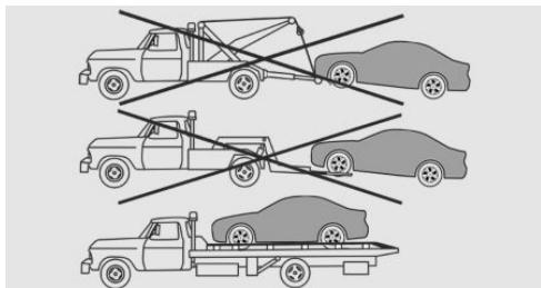
The vehicle should only be transported on a loading platform.
