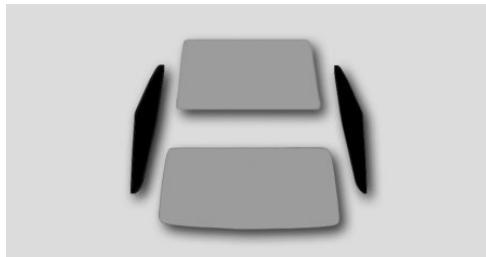
If the roller sunblind on the display is touched again while the roller sunblind is moving, it will move in the opposite direction.
