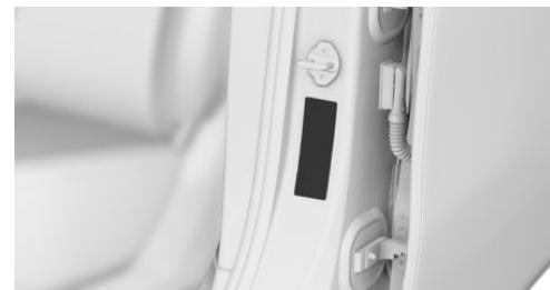
These pressure values can also be found on the tire pressure label on the driver's door pillar.
