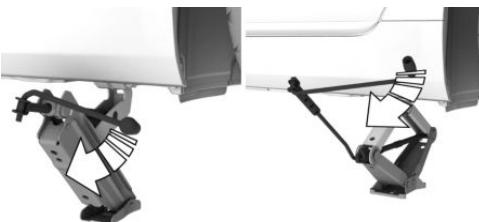
4. Take your hand away from the jack as soon as the jack is under load and continue turning the jack crank handle or lever with one hand.
