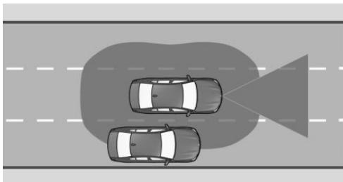
Radar sensors monitor the space next to the vehicle when traveling faster than a minimum speed and up to approx. 130 mph/210 km/h.
