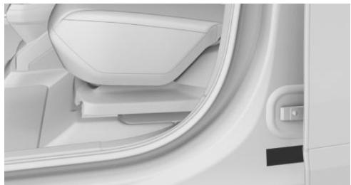
The vehicle identification number can be found on the nameplate, on the left-hand side of the vehicle.
