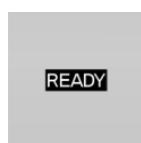
The display in the instrument cluster indicates that the Auto Start/Stop function is ready for an automatic engine start.
