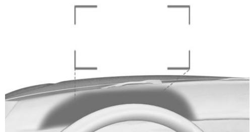
The protective glass of the Head-up display is located between the steering wheel and the windshield.
