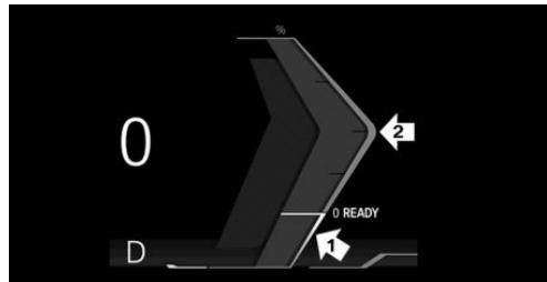
Needle in range of arrow 1: display for energy recovery such as while decelerating CHARGE.
