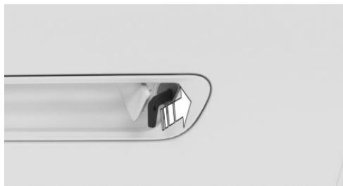
4. Remove the integrated key from the door lock.
