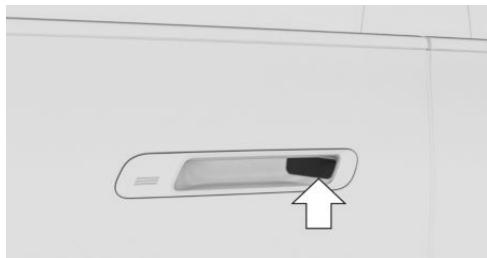
2. Slide out the integrated key at the open side of the vehicle key.
