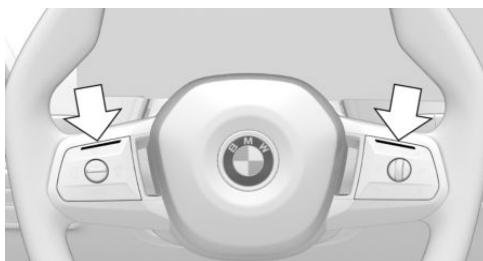
The two LEDs above the keypads light up depending on the situation.
