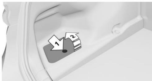
Turn the screw cap in the cover by 90°, arrow 1, and fold down the trim panel, arrow 2.
