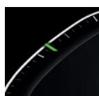
A mark is displayed on the speedometer for the set speed.
