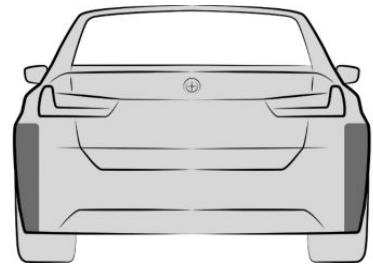
The radar sensors are located on the side in the rear bumper.
