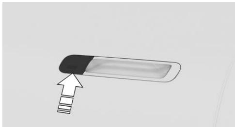
Hold the near field communication antenna of the smartphone directly and centered on the external door handle of the driver's door. The
