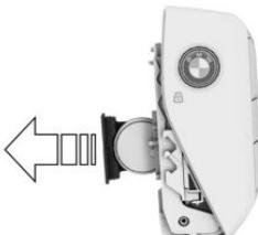
3. Remove the battery from the battery housing.
