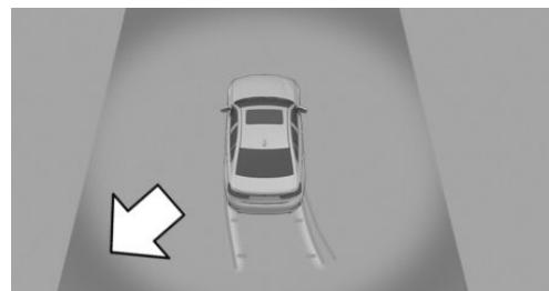
In the Park Distance Control view, the respective boundary area flashes red if vehicles are detected by the sensors.
