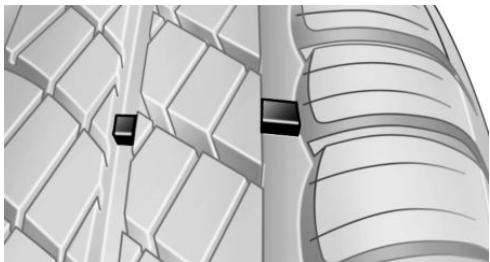
Distributed over the tire circumference are the tire manufacturer's wear indicators with a height of at least 0.06 in/1.6 mm, which serve as an indicator of tire tread wear.
