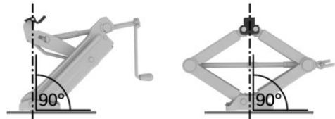
6. Make sure that the car jack foot is vertical and at a right angle beneath the jacking point after extending the vehicle jack.
