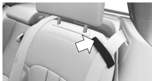
When fastening the safety belts on the rear seats, make sure that the belt loop is closed.
