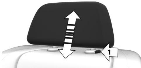
The height of the outer head restraints can be adjusted.
