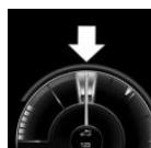
The mark in the consumption display is located at the zero point and is backlit in blue.
