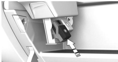
7. Push the cartridge holder up, until it engages. Make sure that no objects press against the cartridge holder from below, otherwise the function of the ambient air package could be impacted.
