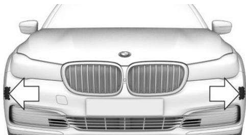
Depending on the vehicle equipment, two additional radar sensors are located in the front bumpers.
