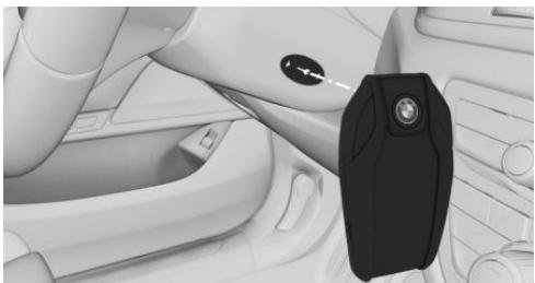
It is not possible to switch on the drive-ready state if the display key has not been detected.
