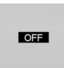
OFF is displayed in the instrument cluster. The drivetrain is switched off and standby state switched on.
