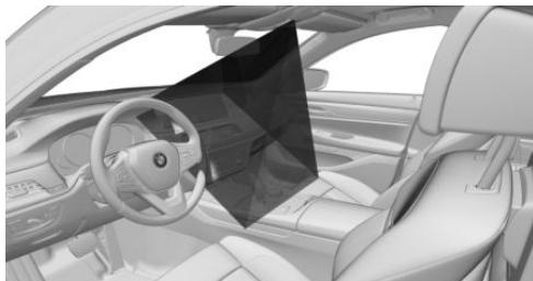
The gestures that are performed underneath the interior mirror are captured by a camera in the roofliner.
