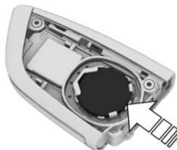
4. Insert a type CR 2032 battery with the positive side facing up.
