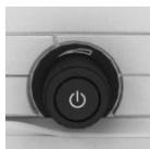
Press and hold the button until the OFF indicator on the instrument cluster goes out.
